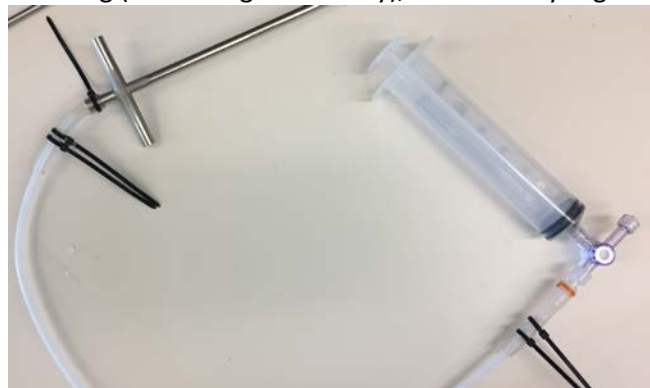
Assembled set-up for pushpoint sampling.
