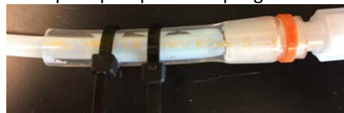
Close up of Teflon-to-tygon-to-3-way valve sampling port. Note that the Teflon tubing is pushed all the way to the luer lock connector. The tygon tubing is secured to the Teflon tubing with zip ties.
