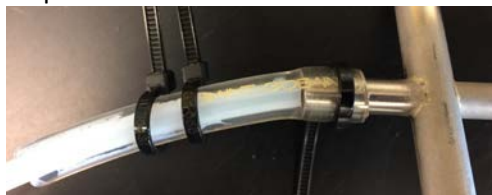
Close up of Teflon-to-tygon-to-pushpoint connections. Note that the Teflon tubing is pushed all the way to the pushpoint opening. The tygon tubing is secured to the Teflon tubing and to the pushpoint with zip ties.
