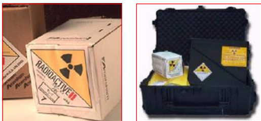
Figure 3-2. Examples of Packaged Radioactive Materials
