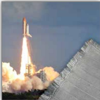
**1989** Advanced ceramic fabric materials developed at PNL helped in space exploration. Ceralite™ materials, made from continuous fibers of metallic oxides or other low-density materials, were used on space shuttle flights to significantly reduce the mass and weight of heat radiators, piping, and other spacecraft components.
