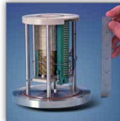
**1999** The award-winning Electrodynamic ion Funnel designed at PNNL significantly improved the sensitivity of certain mass spectrometry tools and other analytical instruments. Mass spectrometry is used in environmental, biotechnology and drug applications, as well as in medical, biological and other broad areas of research.
