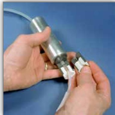
**1983** The award-winning Portable Blood Irradiator developed at PNL is the first fully portable device for continuous irradiation of blood. The device showed promise in suppressing early rejection of organ and tissue transplants by continuously irradiating a patient's blood.
