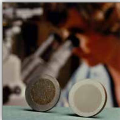
**1982** PNL designed a glassy, stainless steel coating with corrosive-resistant properties comparable to titanium. The coating could be applied to nearly any metal surface by high-rate, sputter-deposition or electro-deposition. It also could be used in corrosive environments, such as seawater, geothermal wells, nuclear power plants and other chloride liquid environments.
