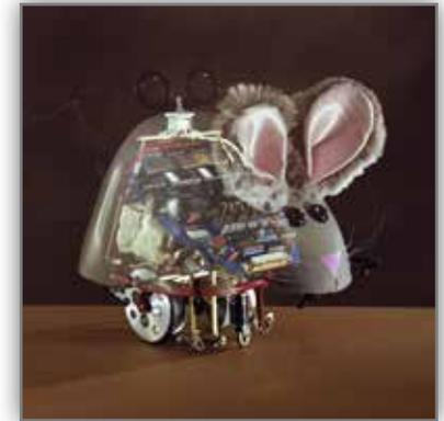
**1978** Micromouse, called "Moonlight Special," took 500 voluntary hours to assemble. It was a self-contained robot that used microprocessor technology to solve complicated mazes.
