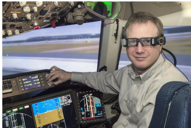
Figure 15. Prototype glasses form factor for commercial aviation HUD. (Source: Arthur, et al., 2015).
