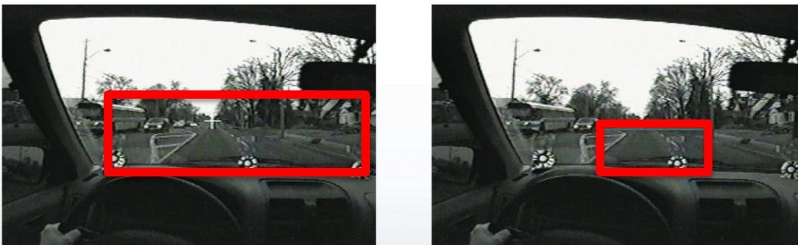
Figure 10. Distribution of eye movements for drivers not using cell phone (left) and when using a hands-free phone (right).
