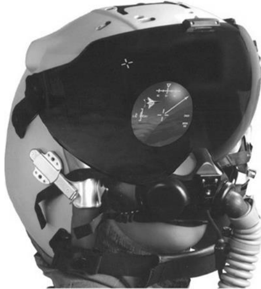
Figure 14. The U.S. Air Force and Navy’s Joint Helmet-Mounted Cueing System. (Source: Foote & Melzer, 2015)
