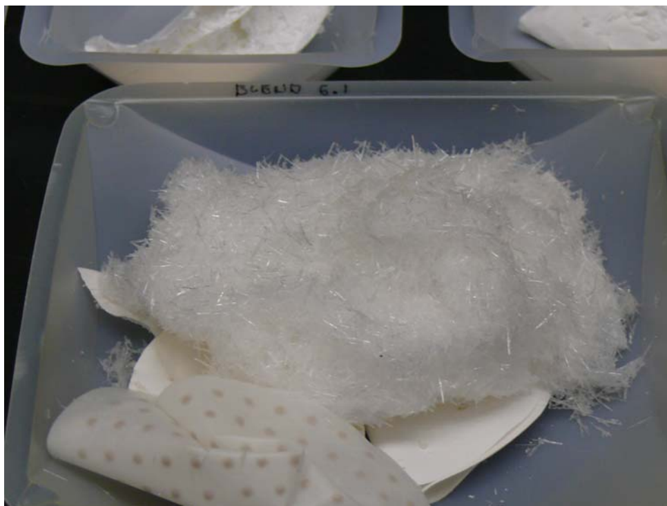
Figure 7.8. Air-Dried Crystals from the 1:1 Wash-Step Permeate: Leachate Mixture
