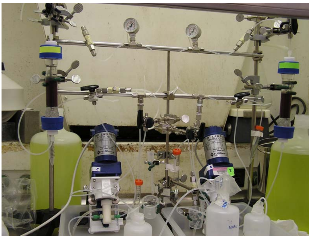
Figure 3.3. Photograph of Two Ion Exchange Column Assemblies, Na-Form Resin (BRF-14 in Yellow Column, left; BRF-15 in Green Column, right)
