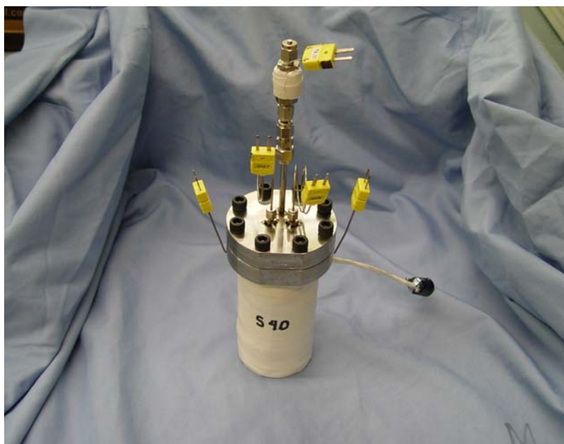
Figure 2.1. Reaction Vessel Used in Small-Scale Gas generation Tests
