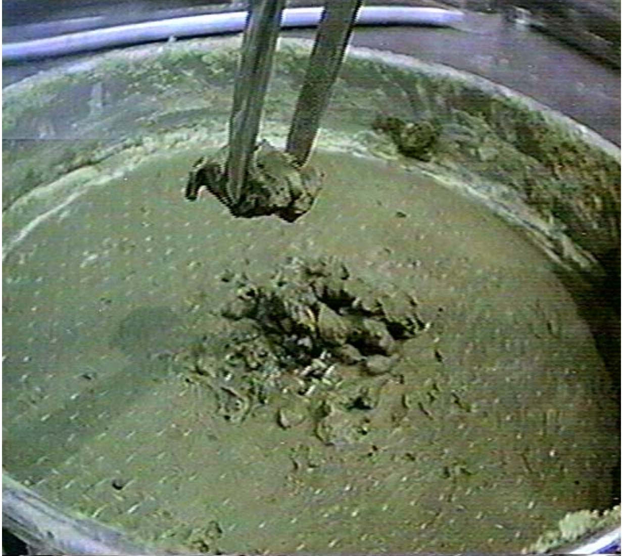
Figure 3.2. Residual Large Particles/Agglomerates Not Forced Through Sieve (Approximately 8 g of a Total of 5251 g Processed)
