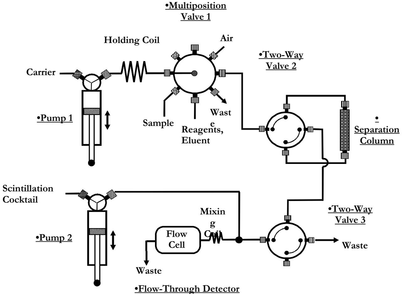
Figure 2.1. Schematic of the Tc Analyzer Instrument
