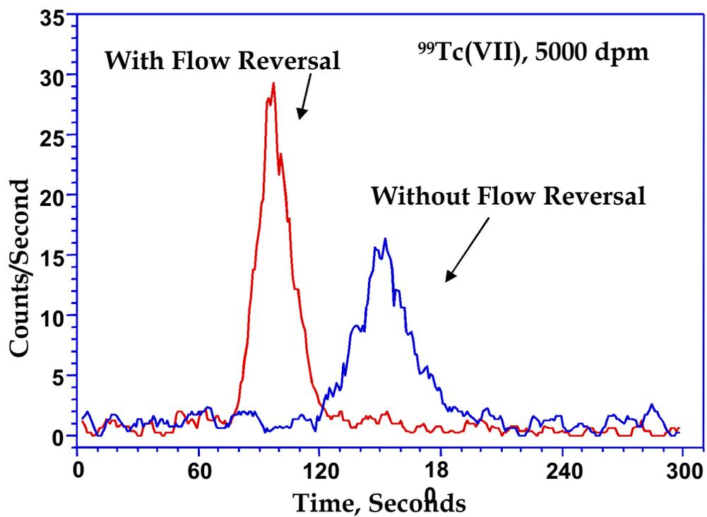
**Figure 3.1.** Tc Elution Profiles With and Without Flow Reversal. Eluent flow rate 1 mL/min. Cocktail flow rate 0.5 mL/min.
