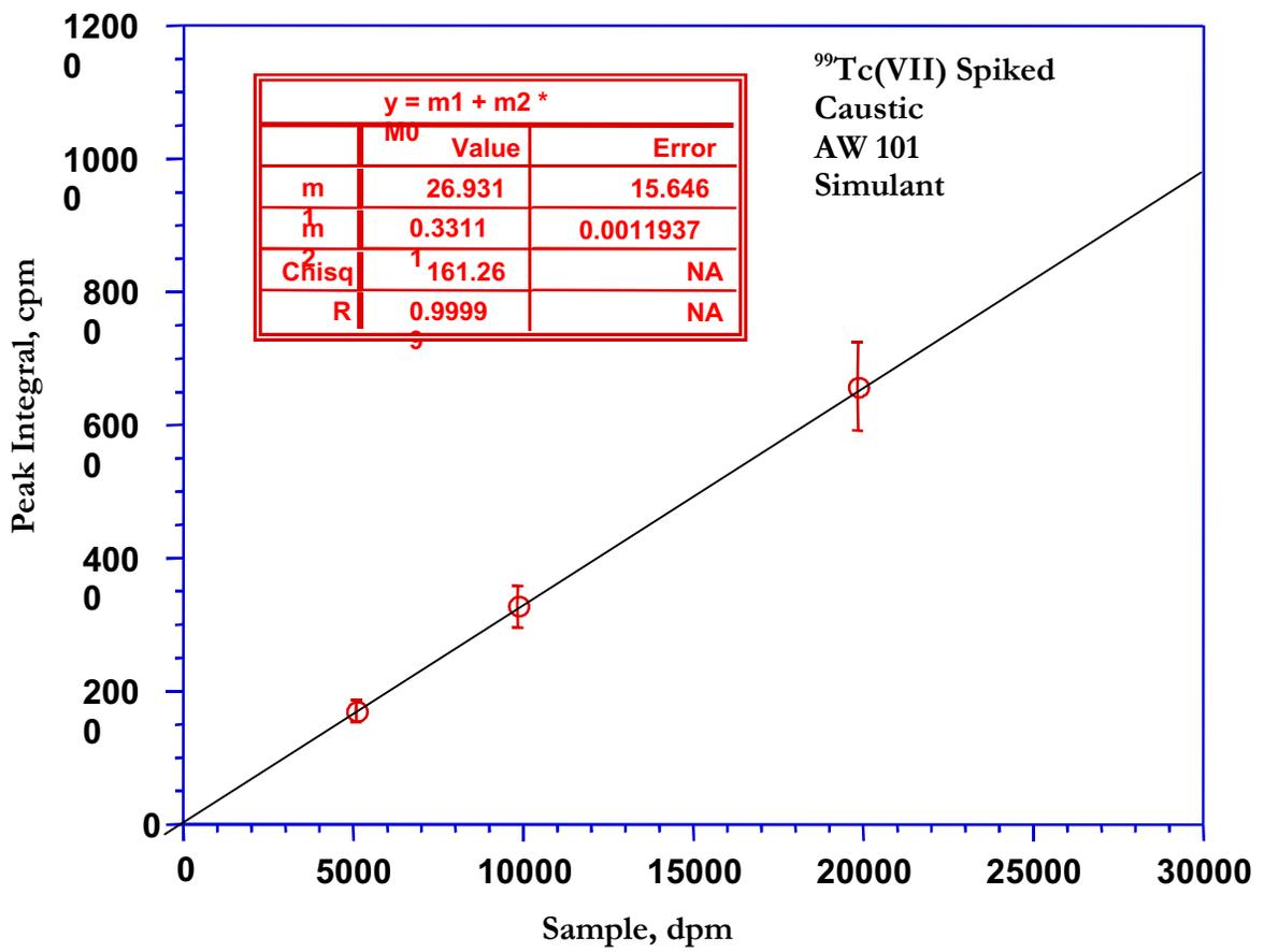
Figure 3.2. Calibration Plot for Analyzing Spiked Caustic Simulant
