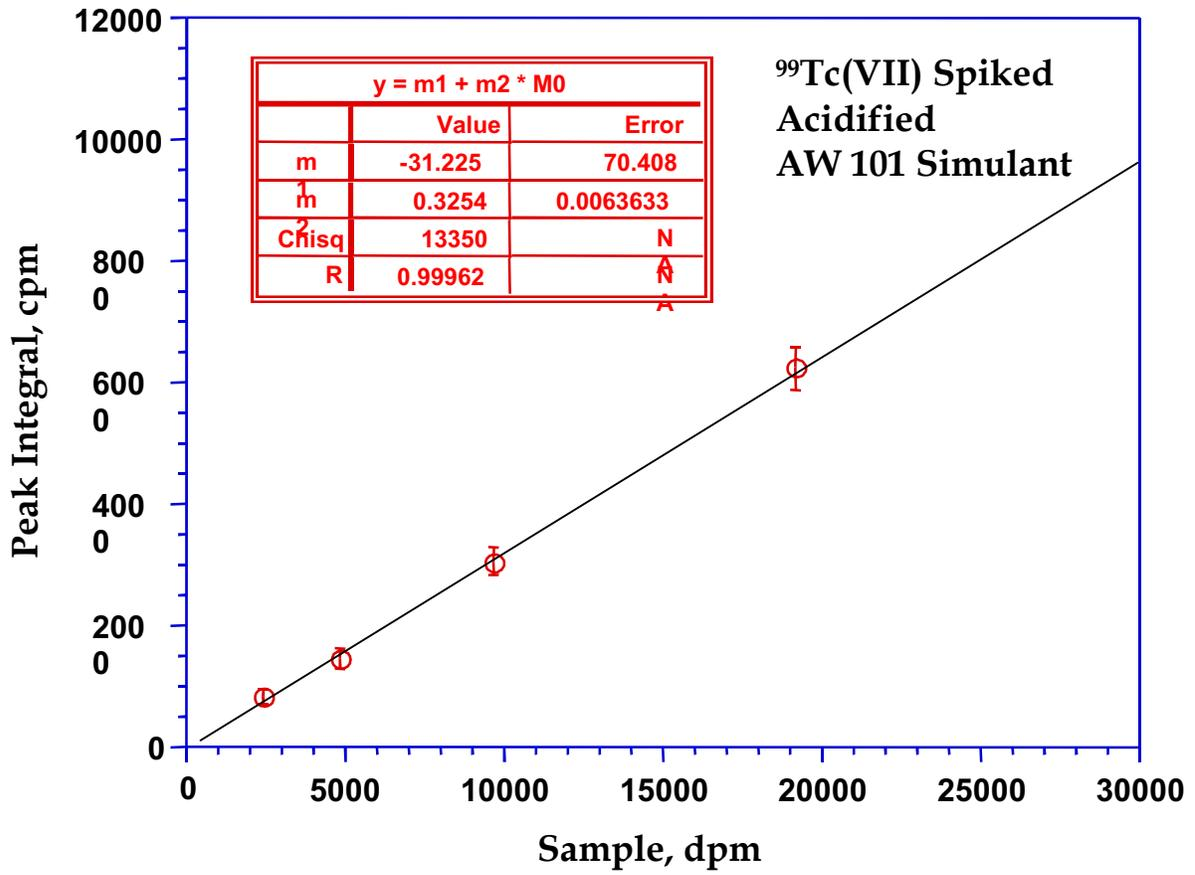
Figure 3.4. Calibration Plot for Analyzing Spiked Acidified Simulant Treated with  $\text{KMnO}_4$
