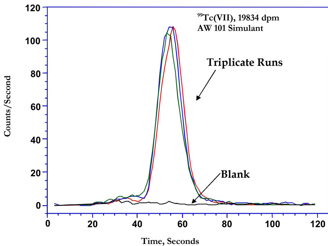
**Figure 3.3.** Detector Traces Corresponding to Triplicate Analyses of the Spiked Caustic Simulant. Eluent flow rate 2 mL/min. Cocktail flow rate 0.5 mL/min.
