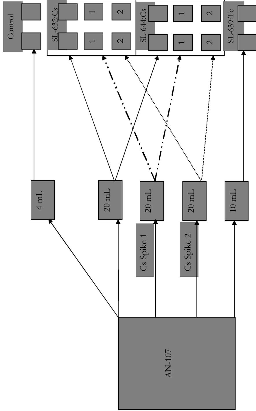
**Figure 2.2** Preparation of AN-107 Cesium and Technetium Spike Solutions and Batch Contacts
