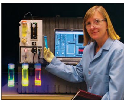
The Biodetection Enabling Analyte Delivery System, or BEADS, developed by PNNL could be used to detect protein signatures including E. coli, salmonella, ricin and other toxins or biological weapons with high specificity and high sensitivity in dirty environments.
