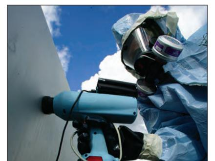
PNNL developed the Acoustic Inspection Device to help identify the contents of sealed containers. For nearly 20 years, PNNL has trained officials from around the world to use this technology and others to help detect materials or components of weapons of mass destruction being shipped across borders.
