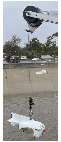
Figure 10. Whole water sampler used in the Los Angeles River.
