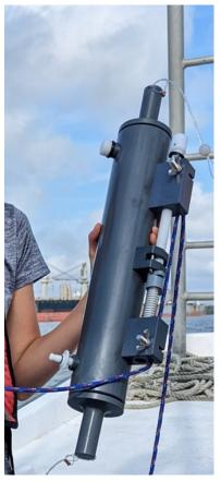
Figure 9. Niskin sampler used in the Mississippi, Columbia, and Delaware rivers.
