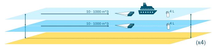
Figure 1. WaterPACT sampling method to collect both net and whole water samples.
