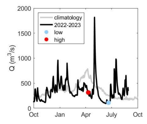
Figure 20. Delaware River climatology, 2022-2023 discharge, and dates for the sampling at the Water Gap site
