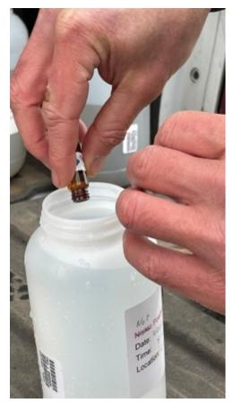
Figure 11. The addition of the spike sample.
