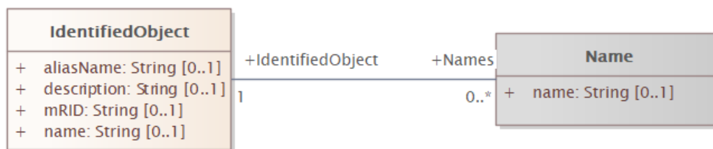
Figure 5: IdentifiedObject class, which is used to specify the unique name and identifier of CIM objects. The Name class should not be used for this purpose.
