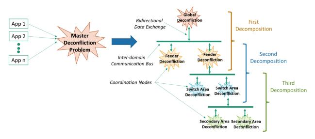
Figure 12: Decomposition iterations of the master deconfliction problem into individual subproblems limited to the controllable devices within each feeder, switch area, and secondary area.
