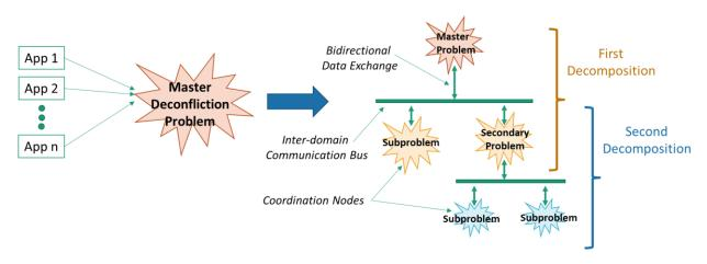
Figure 5: Decomposition of the application deconfliction problem using the Laminar Coordination Framework into subproblems handled by layered coordination nodes.
