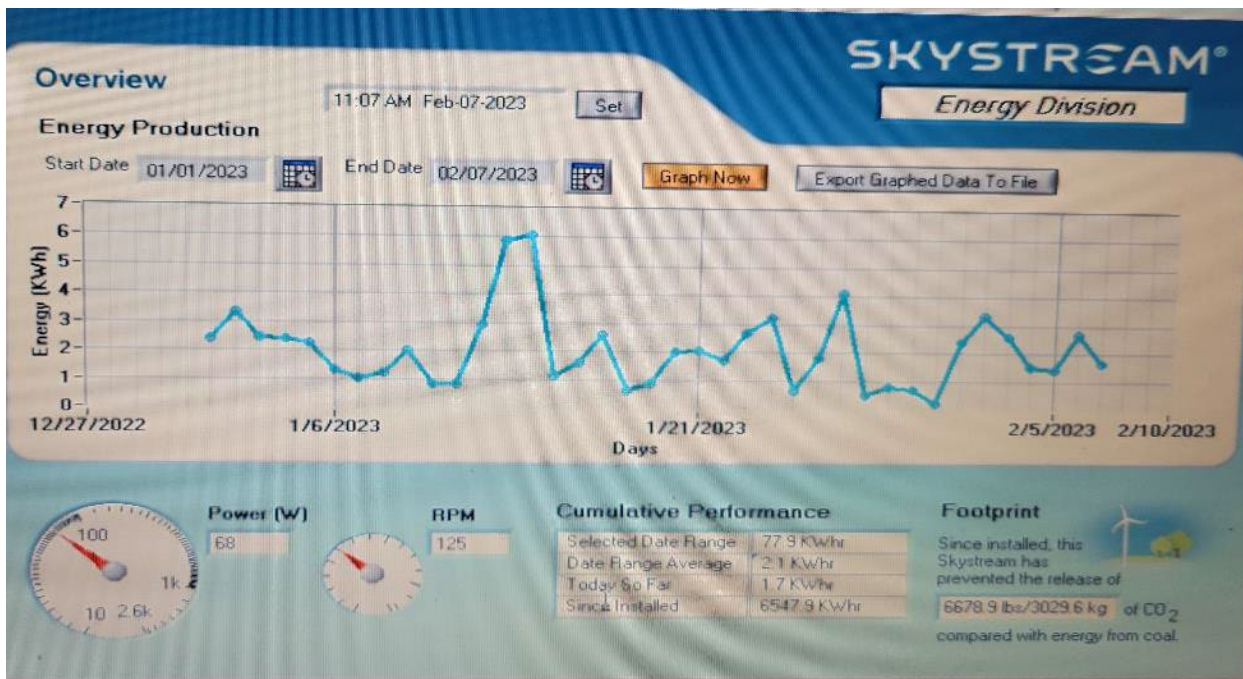
Figure 20. DPW Skystream Wind Turbine January 2023 Power Production Profile
