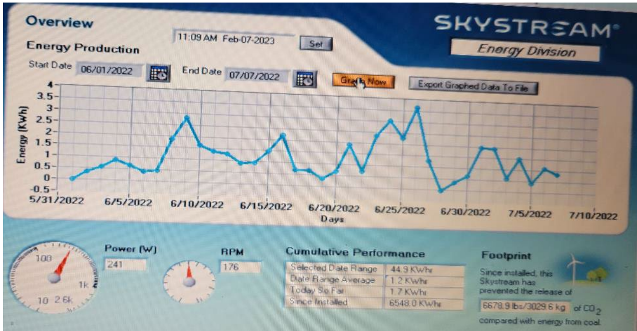
Figure 21. DPW Skystream Wind Turbine June-July 2022 Power Production Profile
