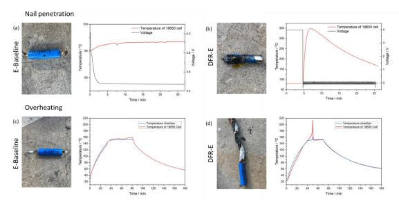
Figure 4. (a) and (b) Photographs (after nail penetration) and temperature/voltage profiles (during nail penetration) of Gr||LFP 18650 cells; (c) and (d) Photographs (after overheating) and temperature profiles (during nail penetration) of Gr||LFP 18650 cells.
