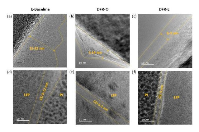
Figure S3. Morphologies of SEIs on Gr formed in (a) E-Baseline, (b) DFR-O and (c) DFR-E, determined by transmission electron microscopy (TEM) after 300 charge/discharge cycles; Morphologies of CEIs in LFP formed in (d) E-Baseline (e), DFR-O and (f) DFR-E determined by TEM after 300 charge/discharge cycles. Note: During sample preparation of LFP slices for TEM characterization, a Pt protection layer was redeposited on the surface of LFP particle so Pt was detected.
