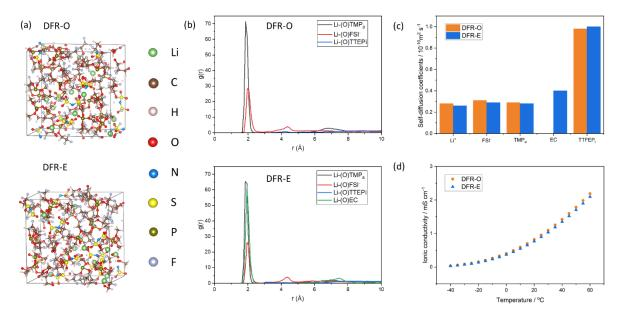
Figure 1. (a) Solvation structures of DFR-O and DFR-E electrolytes obtained by AIMD; (b) RDFs of DRF-O and DFR-E electrolytes obtained from AIMD calculations; (c) self-diffusion coefficients of electrolyte species in DFR-O and DFR-E electrolytes; (d) ionic conductivities of DFR-O and DRR-E electrolytes in the temperature range of -40 to 60 °C.
