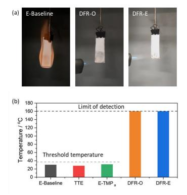
Figure 4. (a) Flammability and (b) flash points of the studied electrolytes determined by ignition tests.
