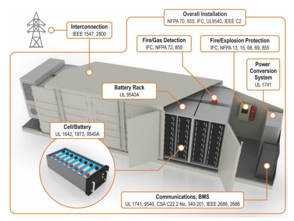
Figure 4-1. Standards Applicable To Stationary BESS Including The Related Safety Standards
