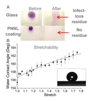
Figure 1: A) Novel water repellent PPE material prevents adhesion of infectious liquids (purple stained bacterial slurry) B) The latex based material exhibits higher hydrophobicity (contact angle) when stretched and causes liquids to bead up and roll off (inset). Bars show standard deviation (N=5).
