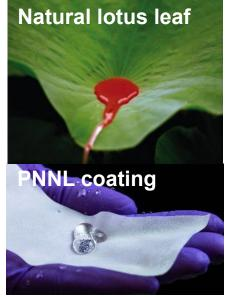
The lotus leaf (top) is naturally superhydrophobic (SHP) and sheds water without residue. A recently PNNL-developed superhydrophobic material (bottom) mimics the texture of the lotus leaf to be water repellant.
