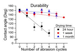
Durability was tested by abrading samples with a known weight (150 g) over sand paper (1000 grit). Coatings given ample time to dry (1 week or more) remained hydrophobic until the underlying latex tore.
