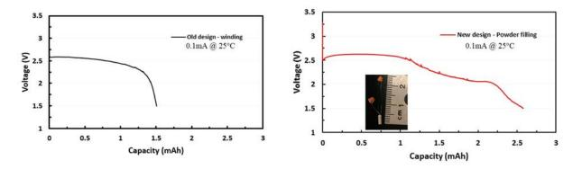
Fig.2 Cell structure and cell performance of Lamprey micro batteries (MB1842) with a) old design (Gen1) and b) new design (Gen2).
