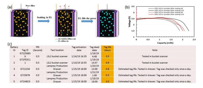
Fig.3 a) Schematic of proposed first solution to create more pores in Gen2 micro battery and b) cell performance from this solution, 10% or 20% LiFSI was used as pore filler. c) Tag life test of 5 asprepared Gen2 MB1842 micro batteries.
