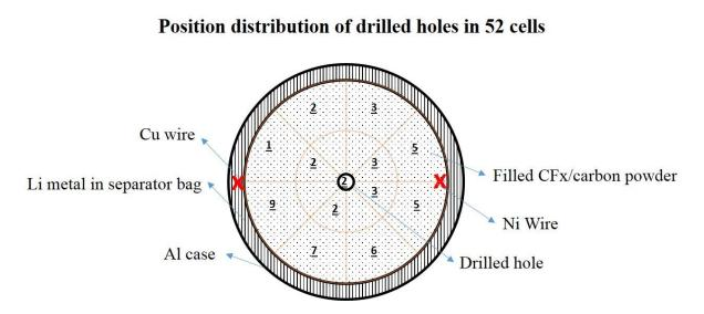
Fig.12 Statistics of the position distribution of the drilled holes in 52 cells during the trial run. Number is the number of cells with drilled hole located in this area.
