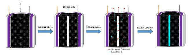
Fig.4 Schematic of proposed second solution to create more pores in Gen2 micro battery.
