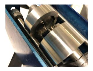
Fig.11 Home-made alignment tools (includes a lift table or lab jack, top and bottom crimping die) for
