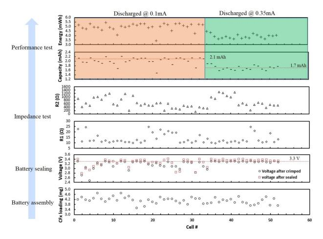
Fig.8 Production data of 1<sup>st</sup> trial run along with the procedure, including 52 MB1842 micro batteries, 33 cells are discharged at 0.1 mA and 0.35 mA for 19 cells.
