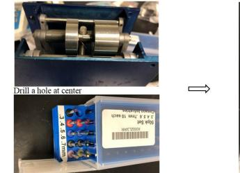
Drill bits, 0.3mm of diameter was used
