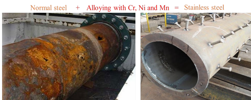
Fig. 1. Pictures of normal steel and stainless steel alloyed with Cr, Ni
