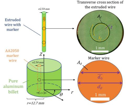
Fig. 2. Geometry and distribution of the 1/3 radius marker before and after FE.
