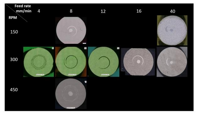
Supplementary data figure 1. Cross-section of friction extrusion wires made with different parameters.
