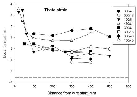
Fig. 7. Theta strain for all eight extrusions. The key indicates the die rotation rate in rpm and the die advance rate in mm/min.
