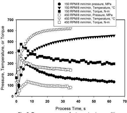
Fig. 3. Process responses for two extrusion conditions.
