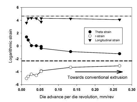
Fig. 9. Average value of each strain component vs. the corresponding die advance per revolution.
