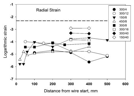
Fig. 6. Radial strain for all eight extrusions. The key indicates the die rotation rate in rpm and the die advance rate in mm/min.
