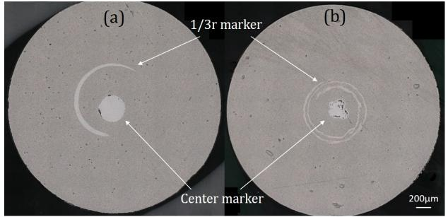
Fig. 4. Etched wire cross sections showing contrast between markers and billets. Both cross sections are from 0.25 m into the respective extrusions. Extrusions made at (a) 150 rpm and 8 mm/min die advance rate, (b) 450 rpm and 8 mm/min.
