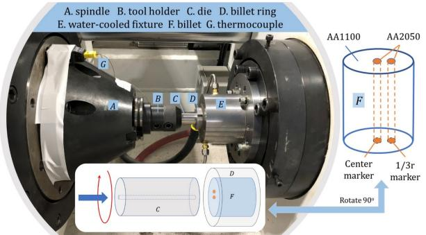
Fig. 1. Experimental setup (left) and schematic of AA1100 billet with inserted AA2050 markers (right).
