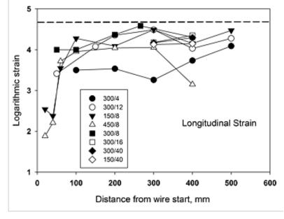
Fig. 5. Longitudinal strain in all eight extrusions. The key indicates the die rotation rate in rpm and the die advance rate in mm/min. The dashed lines indicate the respective strains expected for a "conventional" extrusion with a 10:1 diametral reduction.
