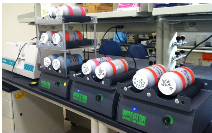
Figure 1. Mixing of soil samples using bench-top rollers.
