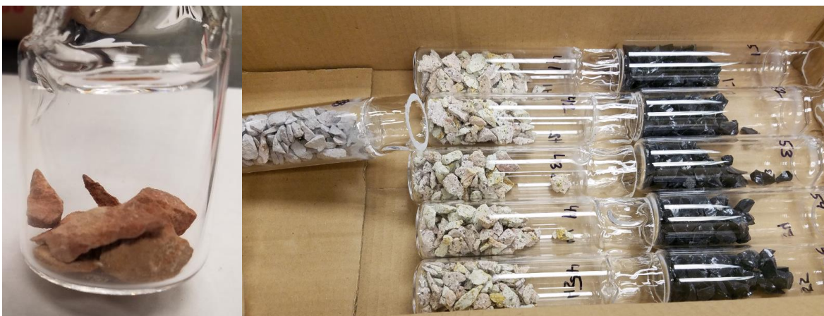
Figure 2. Dolostone sample in a mid-sized ampoule (left) and, from left to right, rhyolite, tuff, and obsidian samples in large-sized ampoules (right).
