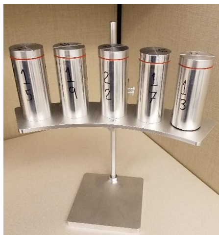
Figure 4. Five mid-sized aluminum canisters, containing a single ampoule each, on the stand used to position the samples around the critical assembly.
