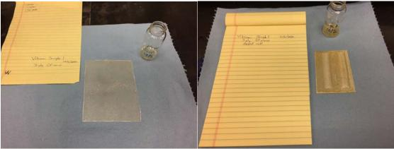
Figure 7. Fiberglass reinforced bio-based vitrimer composites.
