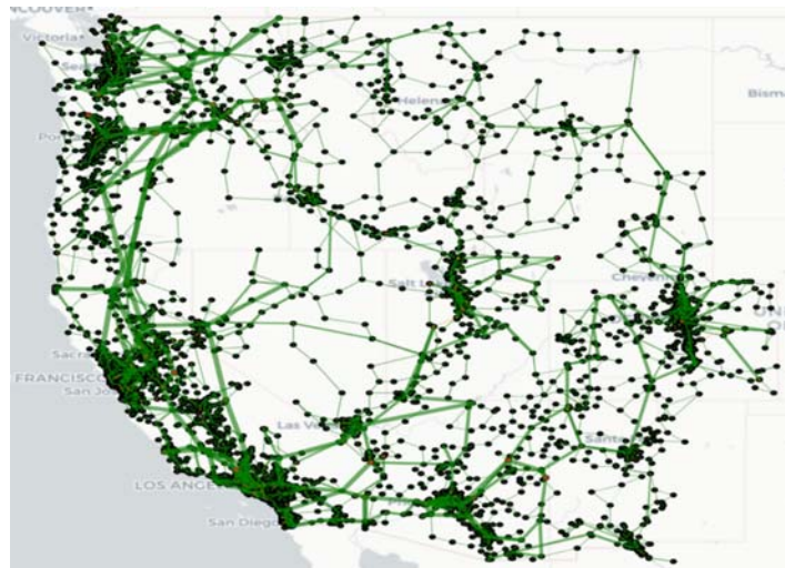
Fig. 2: Topology of the synthetic Western Interconnect from TAMU Electrical Grid Test Repository shows a different connectivity pattern with urban centers and the suburbs having a denser connection.
