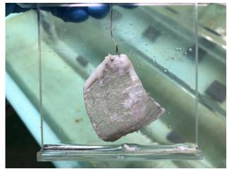
Figure 5 - Photo of the Mg-rich cathode deposit observed in seawater testing.
