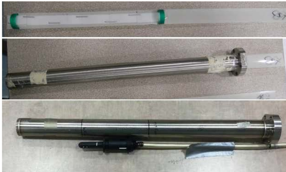
Figure 1: Photos showing LIF film dosimeters stapled to the thin strip of PET with plastic green rings to allow centering within gas vessels (top); a stainless steel gas vessel of 19-mm OD and 26.9-cm length with LIF film assembly inserted (middle); and a Model A1 2S ionization chamber alongside a gas vessel (bottom). Spacers similar to those holding the film strip centered in the vessel, were also applied to the ion chamber.
