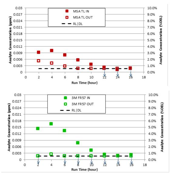
**Figure E.6.** Plots of Measured Formaldehyde Concentrations before the Inlets and after the Outlets of the Two PAPR Cartridges Tested (MSA-TL [TL1] and 3M FR-57 [TL2]). Data points noted with ↓ indicates measurements less than the DL or RL. Outlet data points not visible are obscured by the inlet data points.
