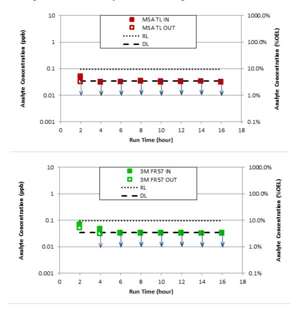
**Figure E.3.** Plots of Measured 2-Pentylfuran Concentrations before the Inlets and after the Outlets of the Two PAPR Cartridges Tested (MSA-TL [TL1] and 3M FR-57 [TL2]). Data points noted with ↓ indicate measurements less than the DL or the RL. Outlet data points not visible are obscured by the inlet data points.
