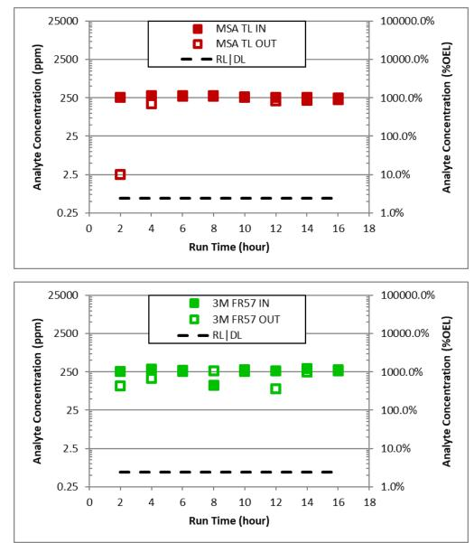
**Figure 7.** Plots of Measured Ammonia Concentrations before the Inlets and after the Outlets of the Two PAPR Cartridges Tested (MSA-TL [TL1] and 3M FR-57 [TL2]) on SX-104. Outlet data points not visible are obscured by the inlet data points.
