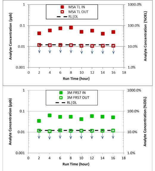
**Figure 12**. Plots of Measured N-nitrosodiethylamine Concentrations before the Inlets and after the Outlets of the Two PAPR Cartridges Tested (MSA-TL [TL1] and 3M FR-57 [TL2]) on SX-104. Data points noted with ↓ indicate measurements less than the DL or RL.
