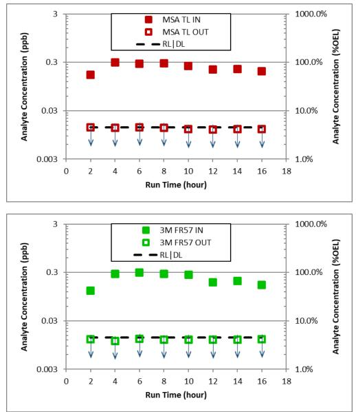
Figure 13. Plots of Measured N-nitrosomethylethylamine Concentrations before the Inlets and after the Outlets of the Two PAPR Cartridges Tested (MSA-TL [TL1] and 3M FR-57 [TL2]) on SX-104. Data points noted with ↓ indicate measurements less than the DL or RL.
