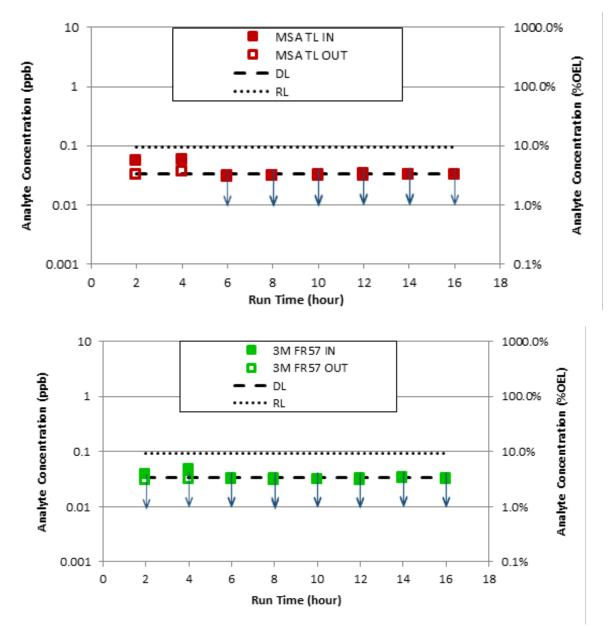
**Figure E.8**. Plot of Measured 2-Pentylfuran Concentrations before the Inlets and after the Outlets of the Two PAPR Cartridges Tested (MSA-TL [TL1] and 3M FR-57 [TL2]). Data points noted with ↓ indicates measurements less than the DL or RL. Outlet data points not visible are obscured by the inlet data points.
