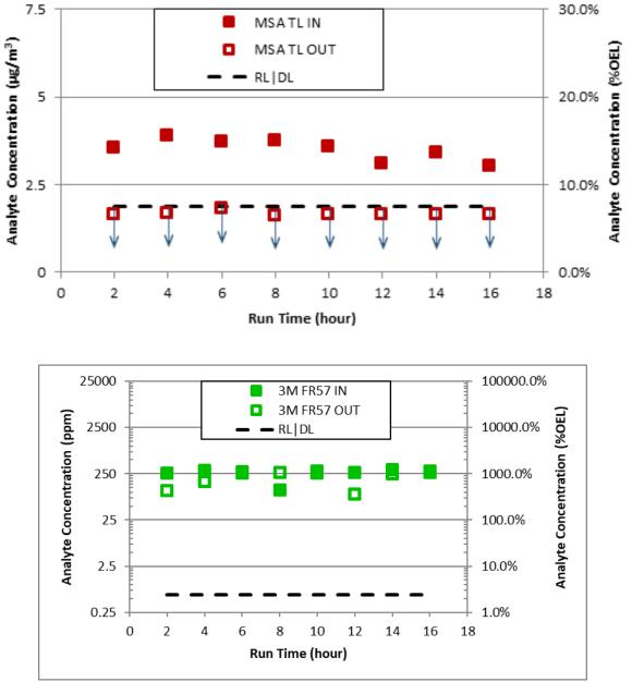
Figure 8. Plots of Measured Mercury Concentrations before the Inlets and after the Outlets of the Two PAPR Cartridges Tested (MSA-TL [TL1] and 3M FR-57 [TL2]) on SX-104. Data points noted with ↓ indicate measurements less than the DL or RL. Outlet data points not visible are obscured by the inlet data points.
