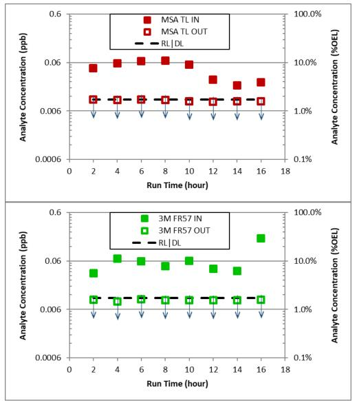
Figure 14. Plots of Measured N-nitrosomorpholine Concentrations before the Inlets and after the Outlets of the Two PAPR Cartridges Tested (MSA-TL [TL1] and 3M FR-57 [TL2]) on SX-104. Data points noted with ↓ indicate measurements less than the DL or RL.
