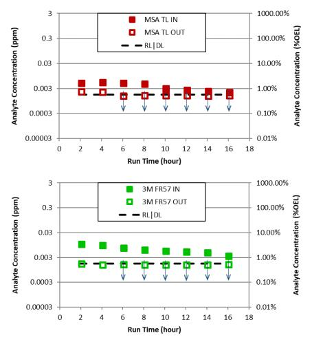
**Figure E.1**. Plots of Measured Formaldehyde Concentrations before the Inlets and after the Outlets of the Two PAPR Cartridges Tested (MSA-TL [TL1] and 3M FR-57 [TL2]). Data points noted with ↓ indicates measurements less than the DL or RL.
