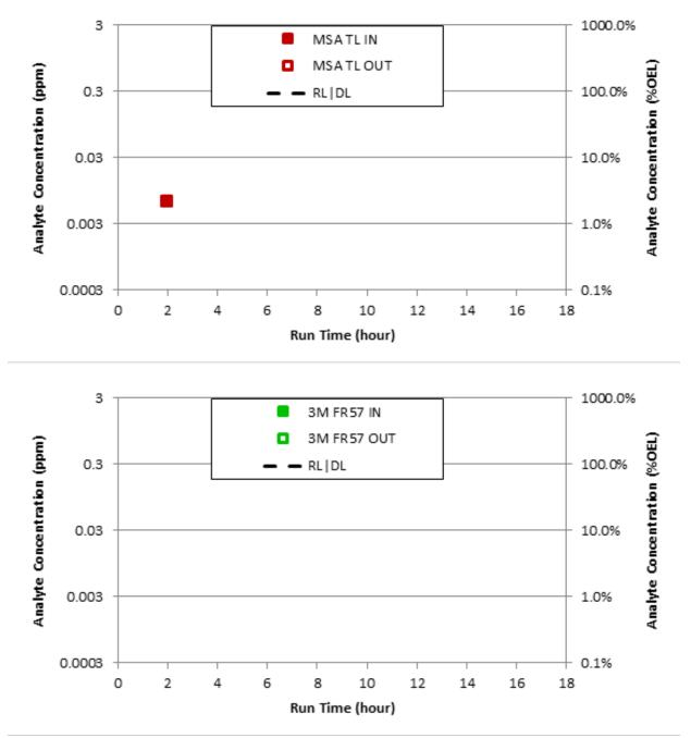
**Figure E.5**. Plots of Measured 2-Nitro-2-methylpropane Concentrations before the Inlets and after the Outlets of the Two PAPR Cartridges Tested (MSA-TL [TL1] and 3M FR-57 [TL2]).
