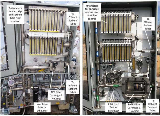
APR Cartridge Test Unit
