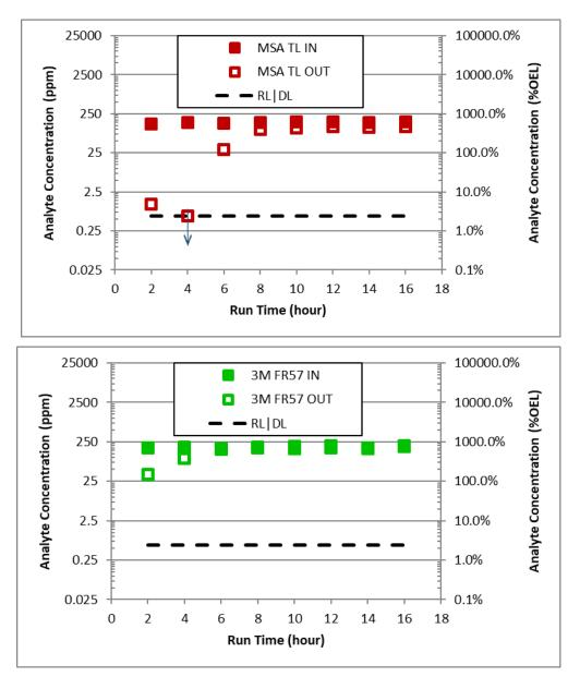
Figure 1. Plots of Measured Ammonia Concentrations before the Inlets and after the Outlets of the Two PAPR Cartridges Tested (MSA-TL [TL1] and 3M FR-57 [TL2]) on SX-101. Data points noted with ↓ indicate measurements less than the DL or RL. Outlet data points not visible are obscured by the inlet data points.
