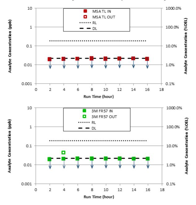
Figure E.2. Plots of Measured 2,3-Dihydrofuran Concentrations before the Inlets and after the Outlets of the Two PAPR Cartridges Tested (MSA-TL [TL1] and 3M FR-57 [TL2]). Data points noted with ↓ indicates measurements less than the DL or RL. Outlet data points not visible are obscured by the inlet data points.
