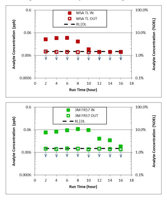
**Figure 6.** Plots of Measured N-nitrosomorpholine Concentrations before the Inlets and after the Outlets of the Two PAPR Cartridges Tested (MSA-TL [TL1] and 3M FR-57 [TL2]) on SX-101. Data points noted with ↓ indicate measurements less than the DL or RL. Outlet data points not visible are obscured by the inlet data points.
