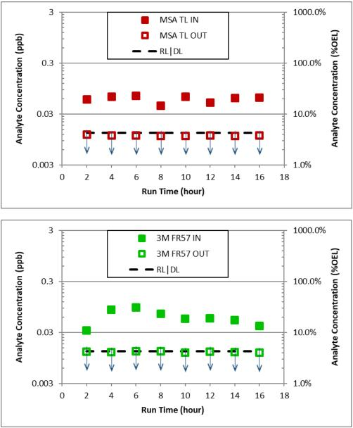
Figure 5. Plots of Measured N-nitrosomethylethylamine Concentrations before the Inlets and after the Outlets of the Two PAPR Cartridges Tested (MSA-TL [TL1] and 3M FR-57 [TL2]) on SX-101. Data points noted with ↓ indicate measurements less than the DL or RL.
