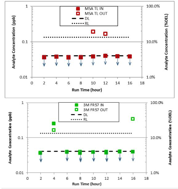
Figure 10. Plots of Measured 2,5-Dimethylfuran Concentrations before the Inlets and after the Outlets of the Two PAPR Cartridges Tested (MSA-TL [TL1] and 3M FR-57 [TL2]) on SX-104. Data points noted with ↓ indicate measurements less than the DL or RL. Outlet data points not visible are obscured by the inlet data points.
