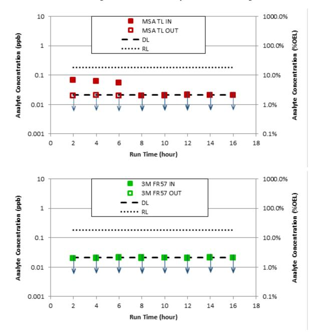
Figure E.7. Plots of Measured 2,3-Dihydrofuran Concentrations before the Inlets and after the Outlets of the Two PAPR Cartridges Tested (MSA-TL [TL1] and 3M FR-57 [TL2]). Data points noted with ↓ indicate measurements less than the DL or RL. Outlet data points not visible are obscured by the inlet data points.
