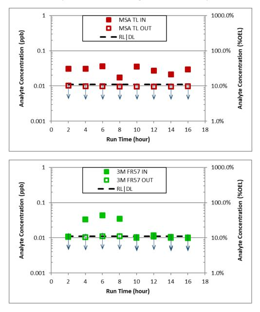
Figure 4. Plots of Measured N-nitrosodiethylamine Concentrations before the Inlets and after the Outlets of the Two PAPR Cartridges Tested (MSA-TL [TL1] and 3M FR-57 [TL2]) on SX-101. Data points noted with ↓ indicate measurements less than the DL or RL. Outlet data points not visible are obscured by the inlet data points.
