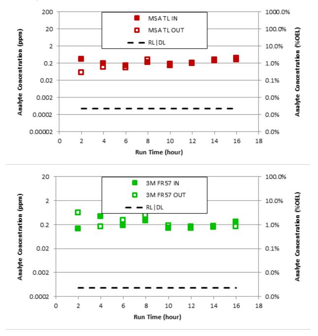
**Figure E.4** Plots of Measured Acetonitrile Concentrations before the Inlets and after the Outlets of the Two PAPR Cartridges Tested (MSA-TL [TL1] and 3M FR-57 [TL2]). Outlet data points not visible are obscured by the inlet data points.
