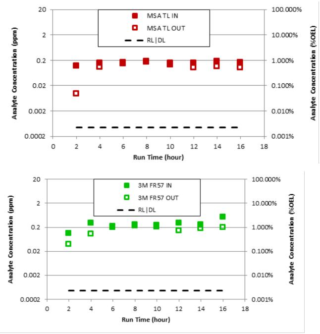
**Figure E.9.** Plot of Measured Acetonitrile Concentrations before the Inlets and after the Outlets of the Two PAPR Cartridges Tested (MSA-TL [TL1] and 3M FR-57 [TL2]). Data points noted with ↓ indicates measurements less than the DL or RL. Outlet data points not visible are obscured by the inlet data points.
