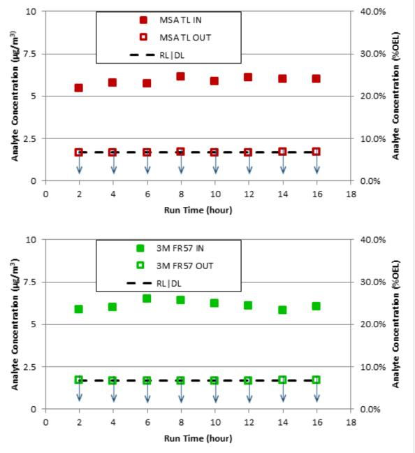
Figure 2. Plots of Measured Mercury Concentrations before the Inlets and after the Outlets of the Two PAPR Cartridges Tested (MSA-TL [TL1] and 3M FR-57 [TL2]) on SX-101. Data points noted with ↓ indicate measurements less than the DL or RL.
