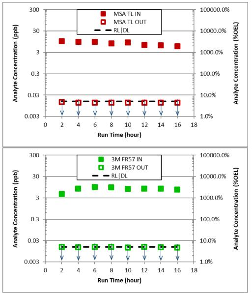
**Figure 3**. Plots of Measured N-nitrosodimethylamine Concentrations before the Inlets and after the Outlets of the Two PAPR Cartridges Tested (MSA-TL [TL1] and 3M FR-57 [TL2]) on SX-101. Data points noted with ↓ indicate measurements less than the DL or RL.
