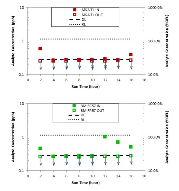
Figure 9. Plot of Measured Furan Concentrations before the Inlets and after the Outlets of the Two PAPR Cartridges Tested (MSA-TL [TL1] and 3M FR-57 [TL2]) on SX-104. Data points noted with ↓ indicates measurements less than the DL or RL. Outlet data points not visible are obscured by the inlet data points.
