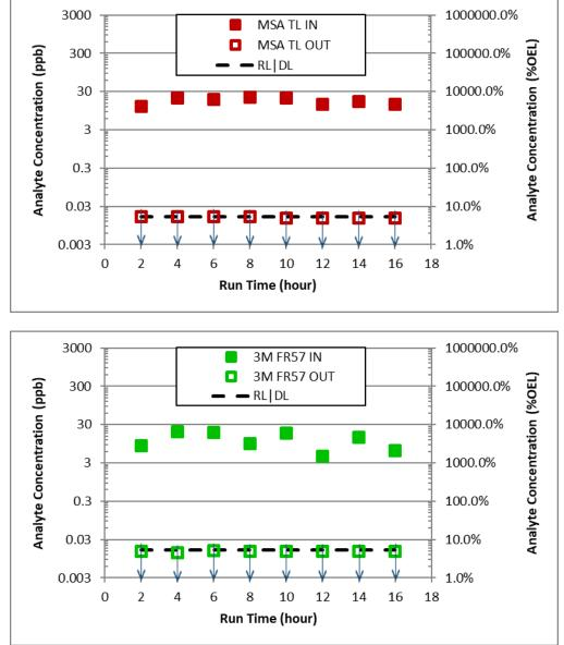
Figure 11. Plots of Measured N-nitrosodimethylamine Concentrations before the Inlets and after the Outlets of the Two PAPR Cartridges Tested (MSA-TL [TL1] and 3M FR-57 [TL2]) on SX-104. Data points noted with ↓ indicate measurements less than the DL or RL.
