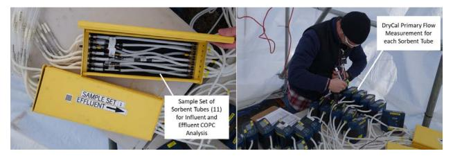
Figure A.3. Photographs of the Sorbent Tube Sampling Test Equipment
