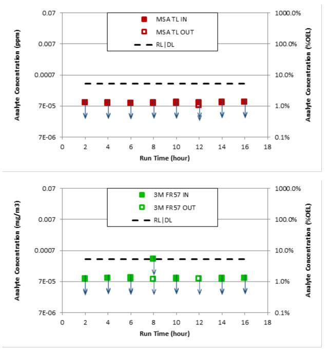
Figure E.10. Plot of Measured Dibutyl Butylphosphonate Concentrations before the Inlets and after the Outlets of the Two PAPR Cartridges Tested (MSA-TL [TL1] and 3M FR-57 [TL2]). Data points noted with ↓ indicates measurements less than the DL or RL. Outlet data points not visible are obscured by the inlet data points.
