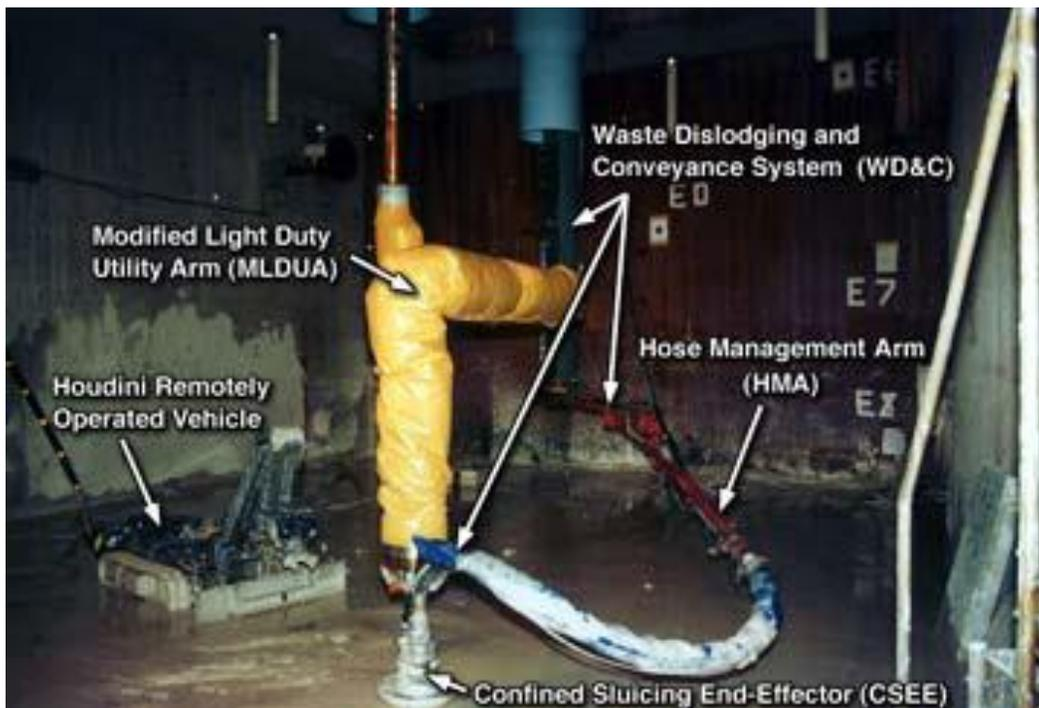
**Figure 2.1.** ORNL GAAT Retrieval In-tank WD&C System with CSEE
