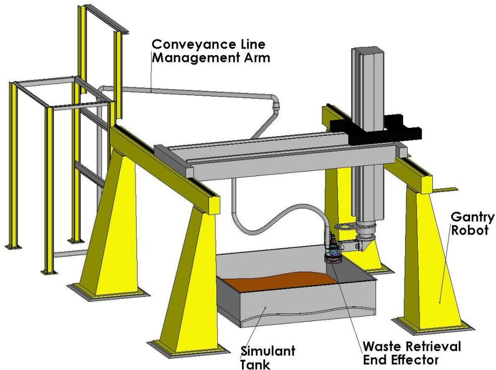
**Figure 4.1.** Hydraulic Test Bed Rendition
