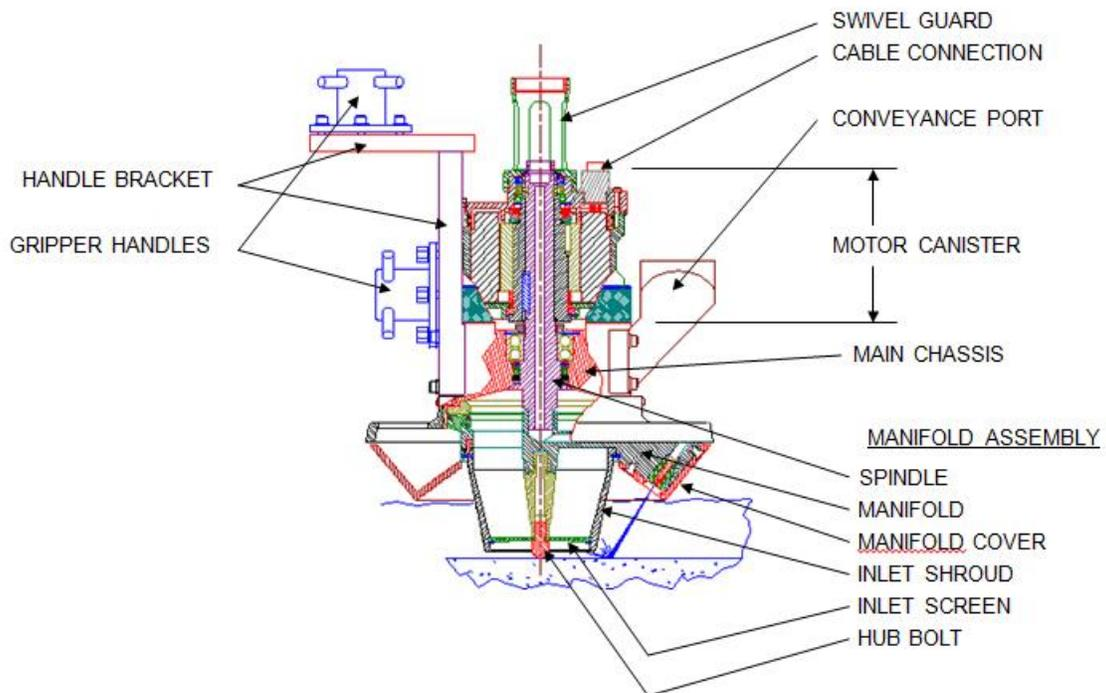
**Figure 2.4.** CSEE Schematic Cross Section Showing Components
