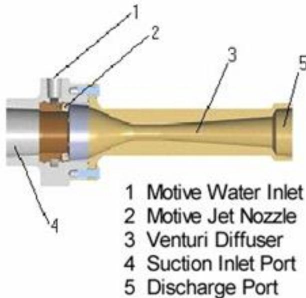
**Figure 2.5.** An Illustration of the Components of the Axial-flow Jet Pump
