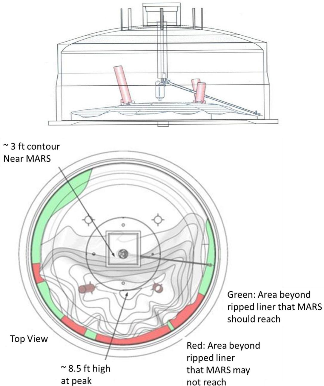
**Figure 3.3.** Example MARS-Vacuum-Bulge Interference and Waste Topology during Retrieval
