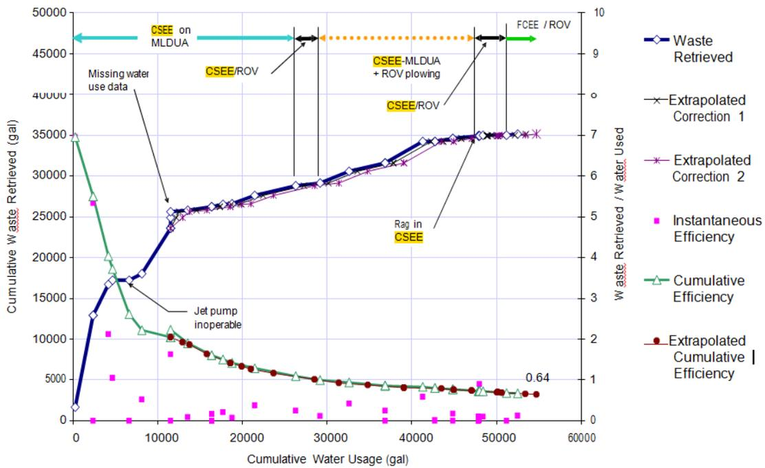
**Figure 2.6.** Waste Retrieval Efficiency for Operations in Tank W-6
