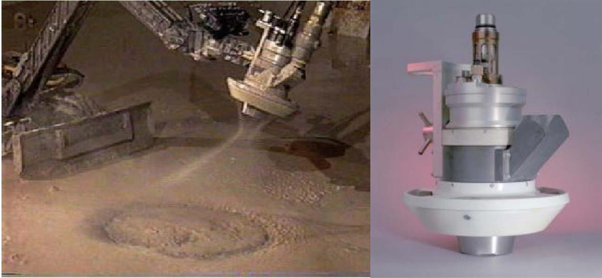
**Figure 2.3.** CSEE Device and Operation View of the CSEE held by Houdini I and Showing the Rotating Cutting Jets Used to Mobilize Waste Material from the GAATs
