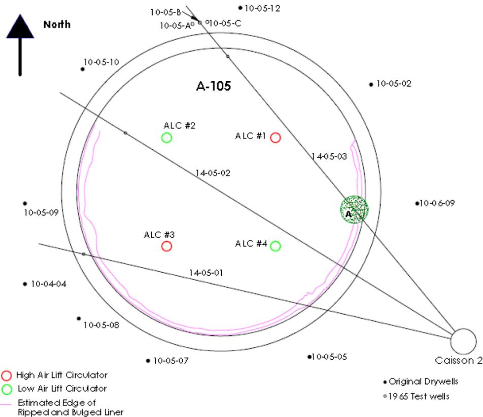
**Figure 3.4.** Tank A-105 Possible Leak Location
