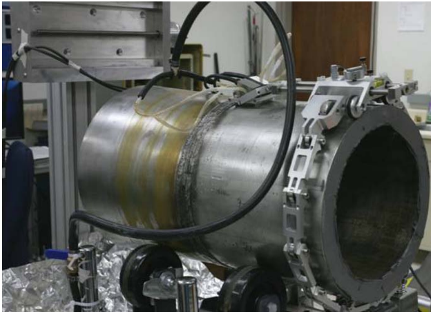
Figure 6.1. Photograph of the DMW Specimen 9C-034 Configured for Standard PA-UT with the ZETEC Manual Scanner Attached Directly onto the Specimen Being Examined
