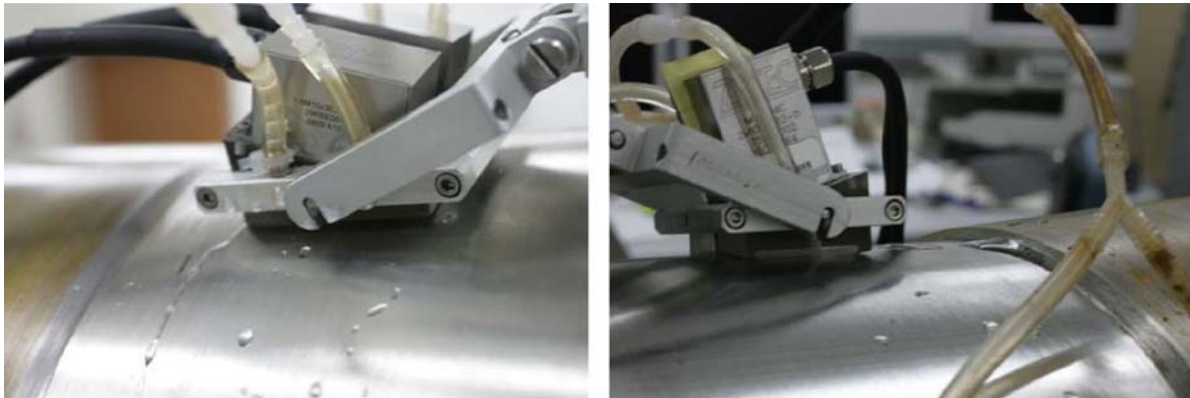
Figure 7.11. Photographs of the OD Surface of DMW Mock-up Specimen 9C-034 after Weld Crown Removal
