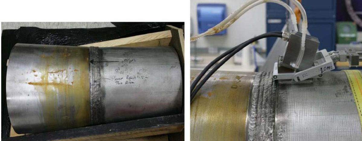
Figure 7.10. Photographs of the Original OD Surface of DMW Mock-up Specimen 9C-034
