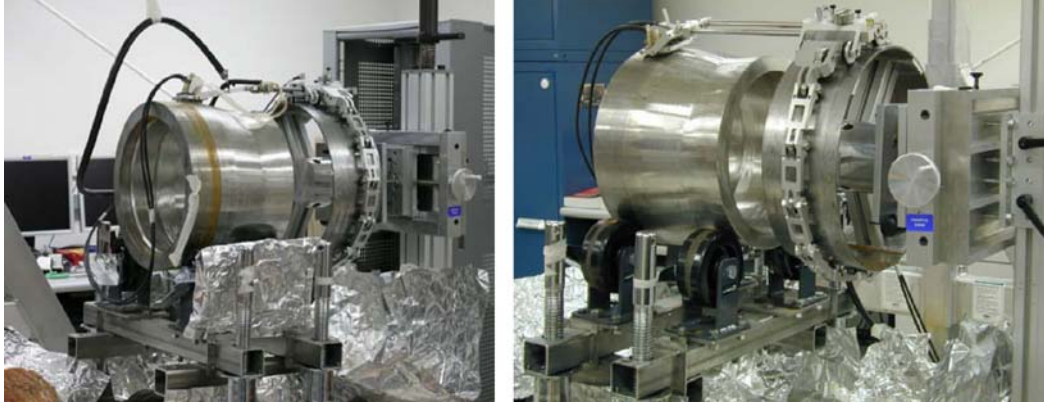
Figure 6.2. Photographs of the DMW Specimen 8C-036. Left: Configured for standard PA-UT with the stainless steel safe end on the right and the carbon steel end on the left side of the photograph. Right: The guide ring, translation slide and floor-to-ceiling brace are shown to the right.
