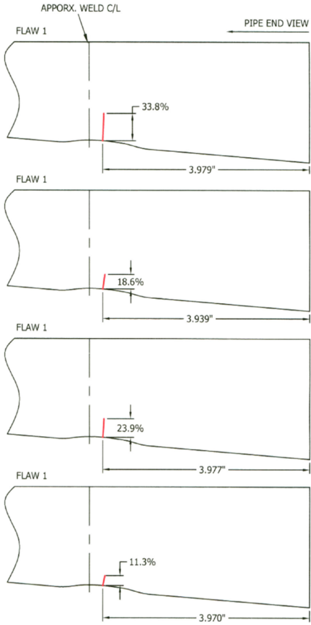
Figure 7.5. Side View Illustration of All Four Thermal Fatigue Cracks Implanted into DMW Mock-up Specimen 9C-023
