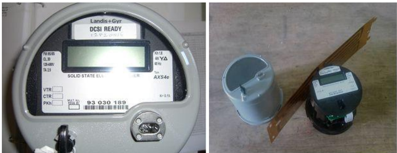
Figure 2.8. MCBH TWACS-Interfaced Commercial Buildings Billing Meter 8 and Transponder
