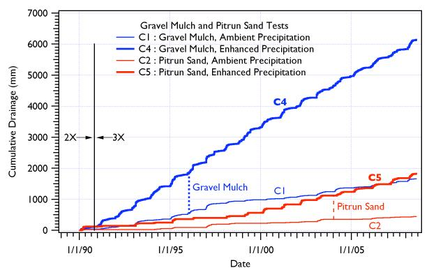
Figure 4.42 FLTF Cumulative Drainage for Treatments C1, C2, C4, and C5
