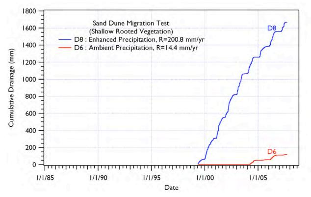
Figure 4.39 FLTF Cumulative Drainage for Treatments D6 and D8 (R is mean annual drainage rate)
