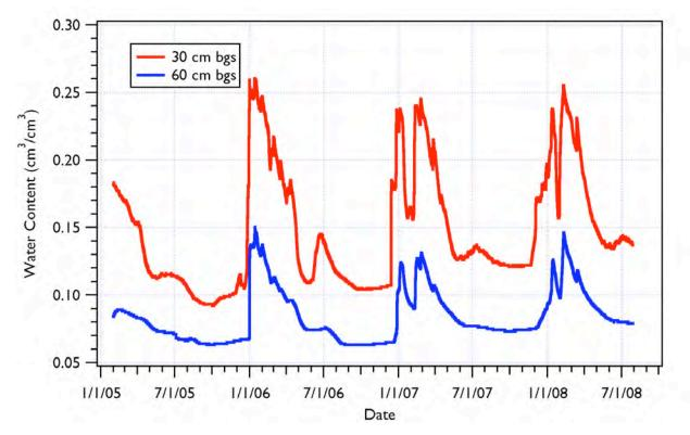
Figure 4.3 Water Content Measured at 30 and 60 cm bgs at the Grass Site
