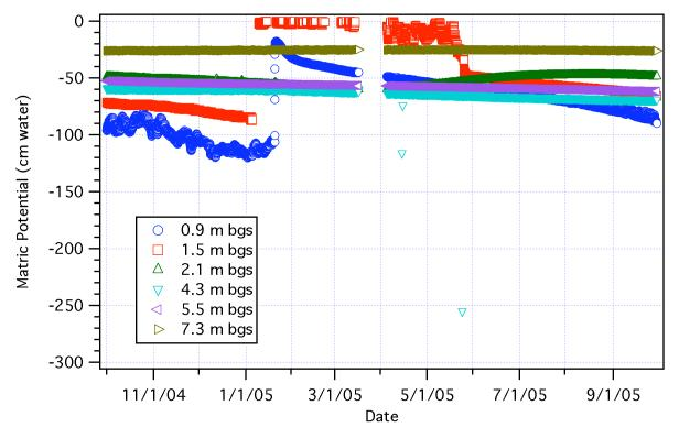
Figure 4.10 300N Lysimeter Matric Potentials Measured at Six Depth for FY 2005 (unfiltered data)
