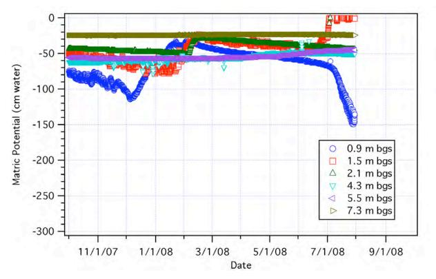
Figure 4.13 300N Lysimeter Matric Potentials Measured at Six Depths for FY 2008 (unfiltered data)
