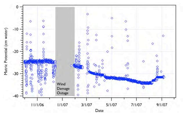
Figure 4.14 300N Lysimeter Cone Penetrometer Tensiometer Matric Potentials at 7.5 m bgs for FY 2007 (unfiltered data)
