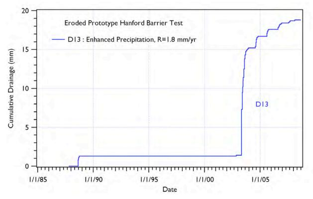
Figure 4.41 FLTF Cumulative Drainage for Treatment D13 (R is mean annual drainage rate)
