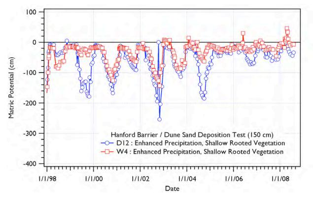
Figure 4.44 FLTF Matric Potentials for Hanford Barrier Dune Sand Deposition Test at Depth 150 cm
