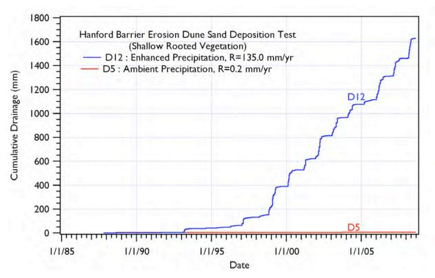
Figure 4.38 FLTF Cumulative Drainage for Treatments D5 and D12 (R is mean annual drainage rate)
