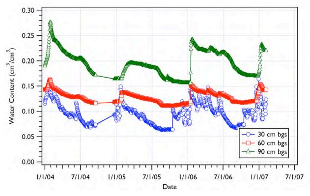
Figure 4.51 SX Pit Measured Water Content at 30, 60, and 90 cm bgs
