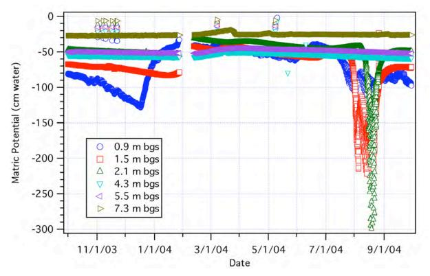
Figure 4.9 300N Lysimeter Matric Potentials Measured at Six Depths for FY 2004 (unfiltered data)
