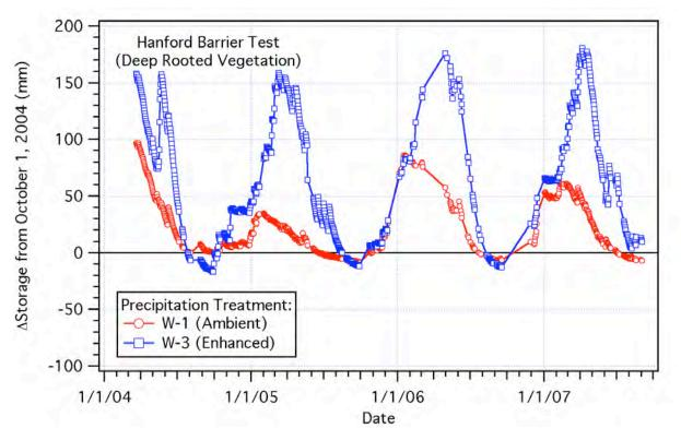
Figure 4.37 FLTF Weighing Lysimeter Treatments W1 and W3 Water Storage Change
