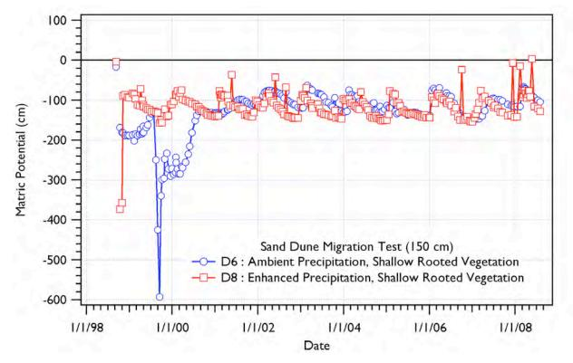
Figure 4.46 FLTF Matric Potentials for Sand Dune Migration Test at Depth 150 cm
