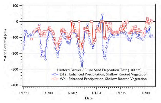
Figure 4.43 FLTF Matric Potentials for Hanford Barrier Dune Sand Deposition Test at Depth 100 cm
