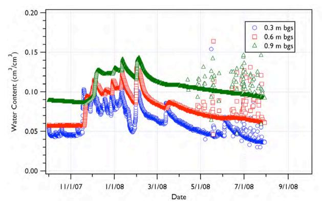
Figure 4.8 300N Lysimeter Water Content Measured at 0.3, 0.6, and 0.9 m bgs for FY 2008
