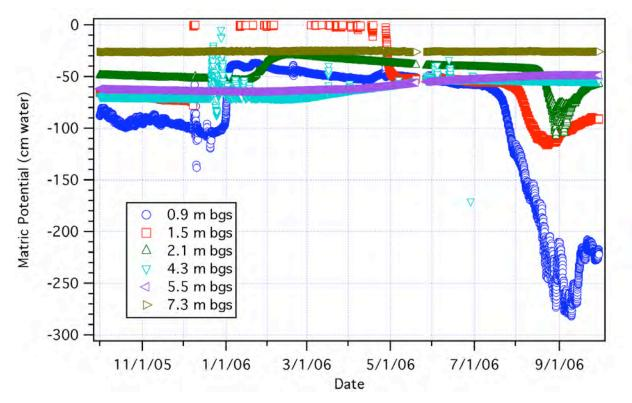
Figure 4.11 300N Lysimeter Matric Potentials Measured at Six Depths for FY 2006 (unfiltered data)
