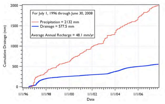
Figure 4.19 SWL Basin Lysimeter Measured Cumulative Drainage
