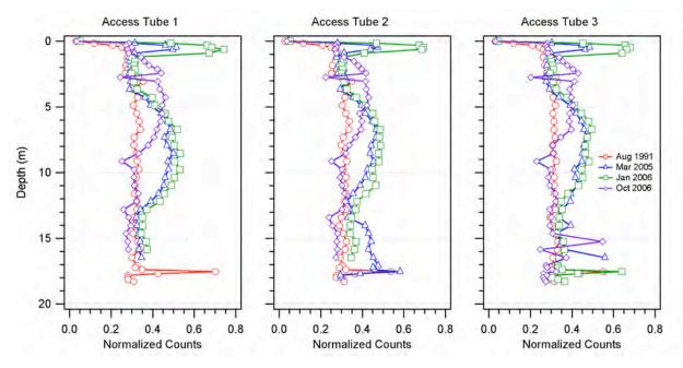
Figure 4.29 200 East Lysimeter Normalized Neutron Probe Counts
