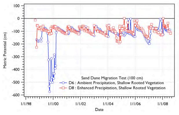
Figure 4.45 FLTF Matric Potentials for Sand Dune Migration Test at Depth 100 cm
