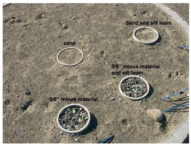
Figure 4.48 Photograph of One of the Four Cement Caissons at the FLTF Pit Showing WFMs Packed with Different Materials
