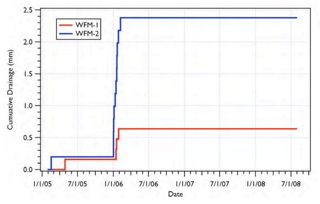
Figure 4.4 WFM Measured Cumulative Drainage at the Grass Site
