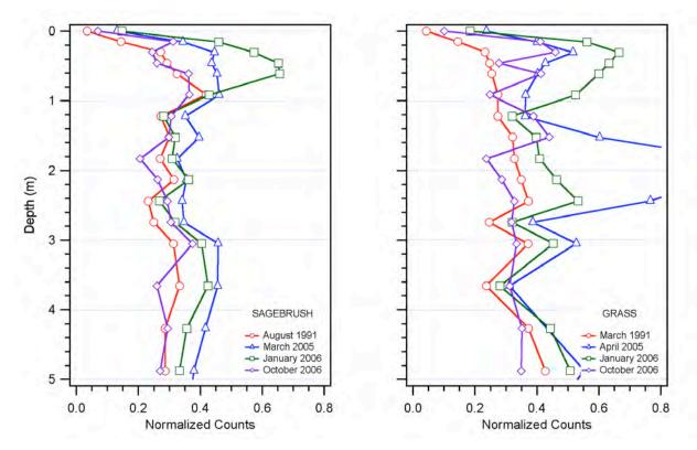
Figure 4.30 200 East Lysimeter Normalized Neutron Probe Counts Taken Under Grass and Sagebrush Vegetative Covers
