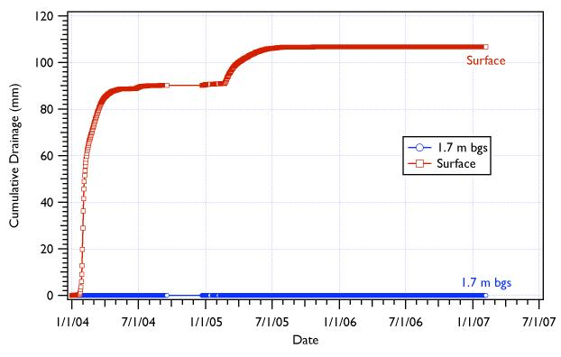
Figure 4.53 SX Pit WFM Measured Cumulative Drainage
