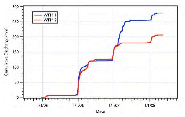
Figure 4.18 SWL Basin WFM Measured Cumulative Drainage
