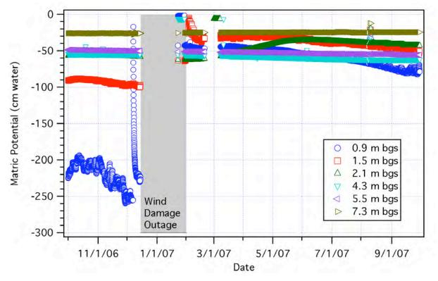
Figure 4.12 300N Lysimeter Matric Potentials Measured at Six Depths for FY 2007 (unfiltered data)
