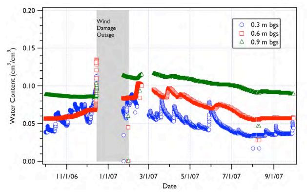
Figure 4.7 300N Lysimeter Water Content Measured at 0.3, 0.6, and 0.9 m bgs for FY 2007
