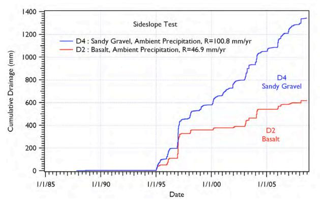
Figure 4.40 FLTF Cumulative Drainage for Treatments D2 and D4 (R is mean annual drainage rate)
