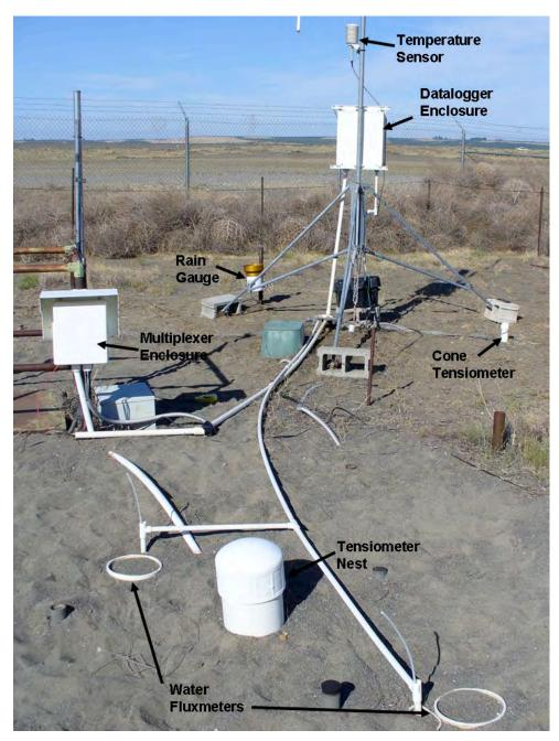
**Figure 4.5** Surface Conditions of 300N Lysimeter Site Shortly After Completion of Site Overhaul (photograph taken September 13, 2007). The coarse textured sand in the foreground is the approximate location of the south caisson.
