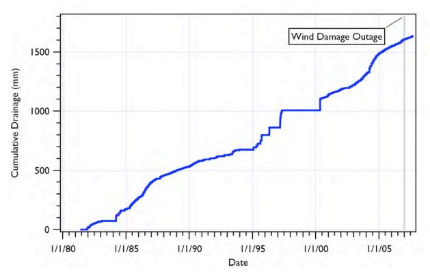
Figure 4.6 300N Lysimeter Measured Cumulative Drainage Since Drainage Onset in 1981
