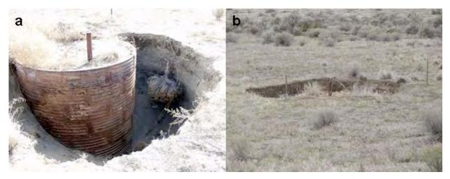
**Figure 4.28** 200 East Lysimeter Subsidence; Image b Shows the Subsidence From a Distance (photograph taken after discovery of soil subsidence in 2005)
