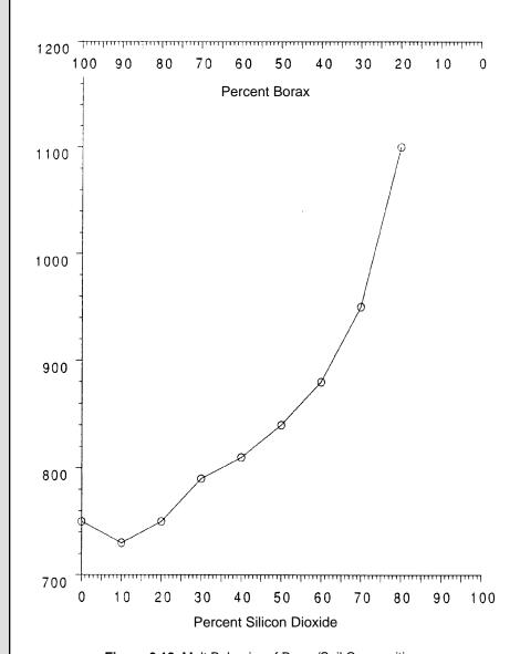
Figure 6.10. Melt Behavior of Borax/Soil Compositions
