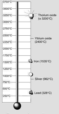
Figure 4.11. Relative Melting Temperatures
