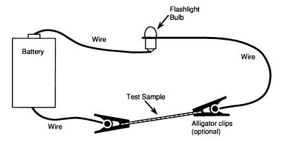
Figure 4.2. Electrical Conductivity Test
