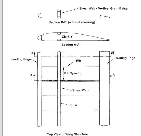
Figure 8.6. Construction Details of a Model Airplane Wing
