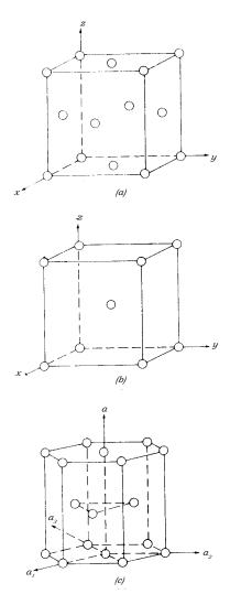
**Figure 5.8**. Crystal Structure of Metals: (a) Face-centered cubic, (b) Body-Centered Cubic, (c) Close-Packed Hexagonal
