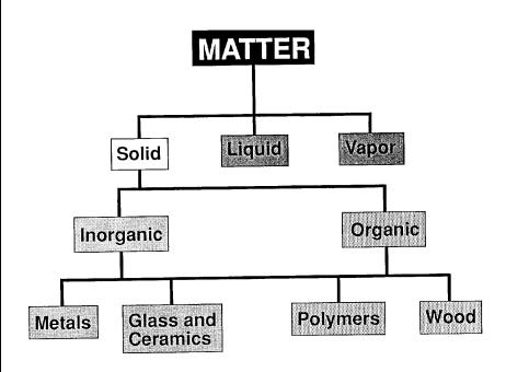
Figure 1.1. Physical Classification of Materials by State
