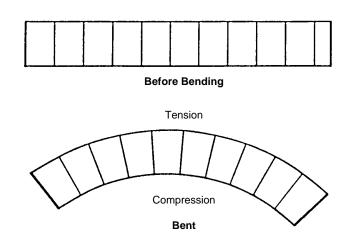
**Figure 8.3.** Foam-Rubber Beam Used to Illustrate Tensile and Compressive Forces Resulting From Bending
