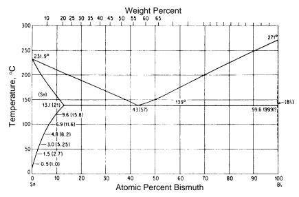
Figure 5.3. Bi-Sn Phase Diagram
