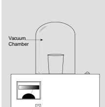
**Figure 7.5**. Vacuum Chamber for De-Airing RTV
