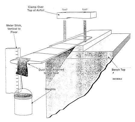
Figure 8.8. Arrangements to Test Stiffness and Strength of Airfoil Sections
