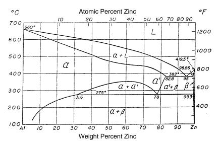
Figure 5.7. Phase Diagram for Aluminum and Zinc
