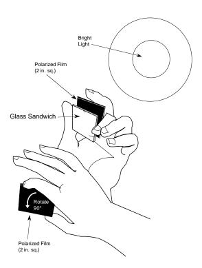
Figure 4.6. Use of Polarized Film for Analyzing Crystal Structures
