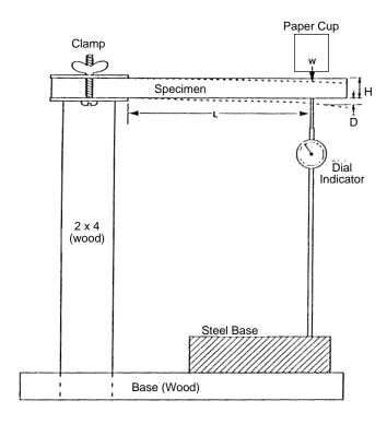
**Figure 8.5.** Apparatus Used to Evaluate Stiffness of Composite Beams by Measuring Deflection of a Cantilever Beam in Bending
