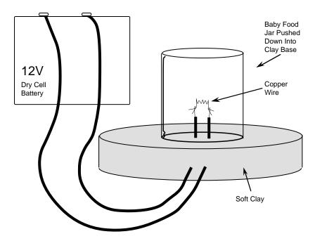
Figure 5.11. Making a Light Bulb
