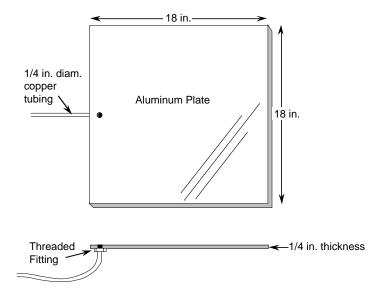
Figure 8.2. Aluminum Vacuum Plate Used in Vacuum Bag Process
