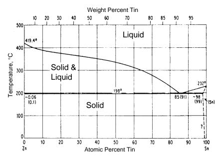
Figure 5.2. Sn-Zn Phase Diagram
