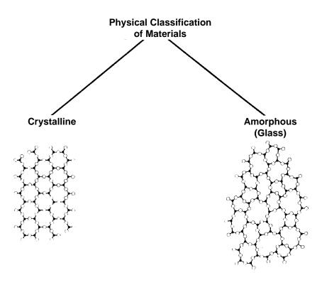
Figure 1.3. Physical Classification of Materials by Atomic Structure
