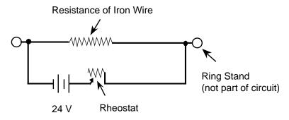
Figure 4.9. Wiring Diagram for Circuit with Batteries
