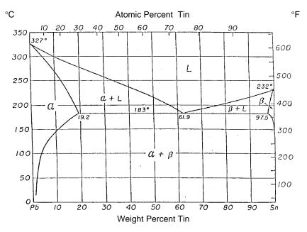
Figure 5.4. Phase Diagram for Tin-Lead Alloys
