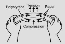
**Figure 8.4.** Two-Faced Reinforced Beam
