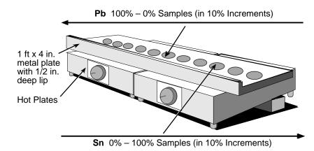
Figure 5.5. Alloying Tin and Lead
