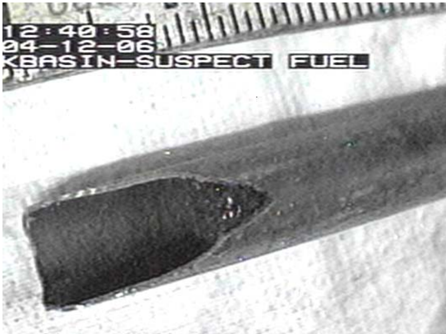
Figure 2.2. Tapered Cut End on SF-4
