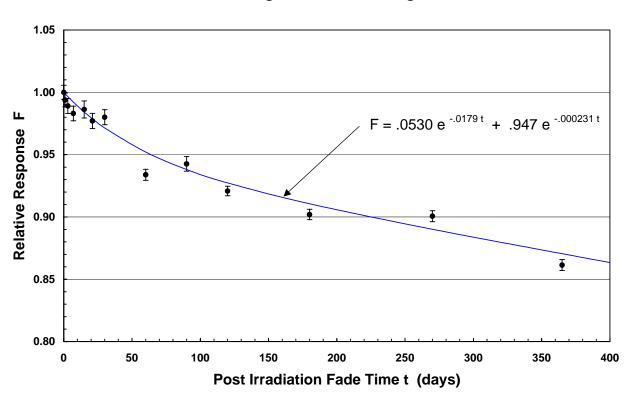
Figure 5.26 Fade Correction for the Hanford Ring
