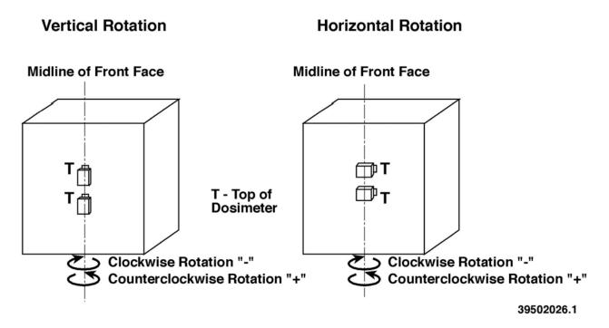
Figure 5.8. Irradiation Setup for Dosimeter Angular Response Evaluation
