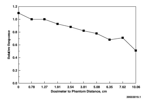
Figure 5.19 Measured Albedo Response of 8816 Neutron Dosimeter
