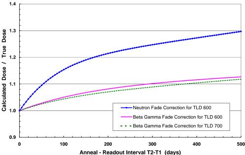
Figure 5.5 Error in default fade correction when entire exposure occurs on last day of use cycle.
