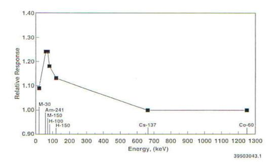
Figure 5.41 Hanford Environmental Dosimeter Energy Response (TLD 700)
