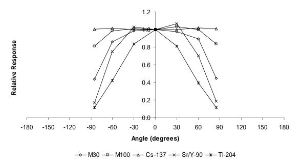
Figure 5.38 EXT-RAD Ring Shallow Dose Angular Response – Horizontal Orientation
