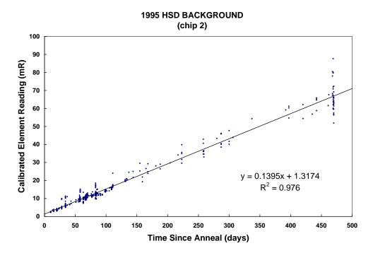
Figure 5.2 Buildup of Environmental Background Signal in HSD Deep Dose Element
