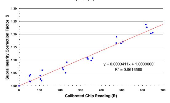
Figure 5.6. Supralinearity Correction for Beta-Gamma Signal in TLD 600 and 700.
