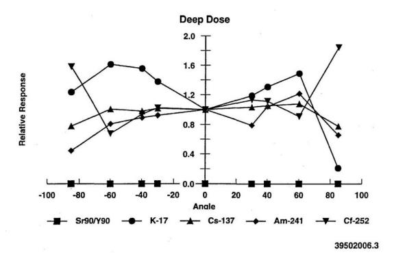
Figure 5.20 Hanford Combination Neutron Dosimeter Angular Response – Horizontal Rotation
