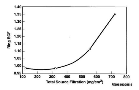
Figure 5.31 Ring BCF vs. 90Sr/90Y Source Filtration
