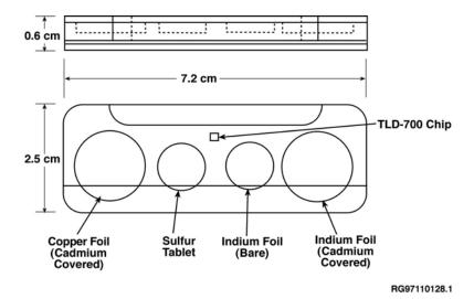
Figure 5.43 Hanford Personal Nuclear Accident Dosimeter
