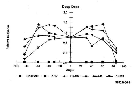
Figure 5.21 Hanford Combination Neutron Dosimeter Angular Response - Vertical Rotation
