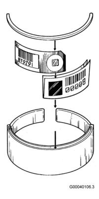
Figure 5.25 Illustration of Hanford Ring Dosimeter
