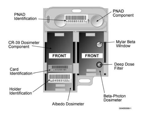
Figure 5.16 Hanford Combination Neutron Dosimeter with PNAD
