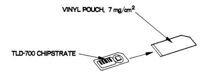
Figure 5.36 Illustration of Chipstrate Sealed in Vinyl Pouch
