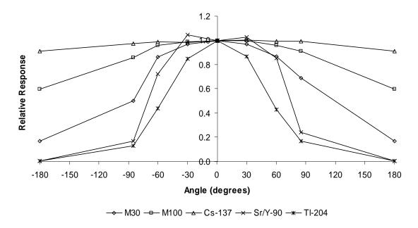
Figure 5.39 EXT-RAD Ring Shallow Dose Angular Response – Vertical Orientation
