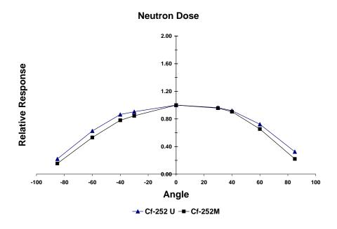
Figure 5.13. HSD Neutron Angular Response – Horizontal Rotation
