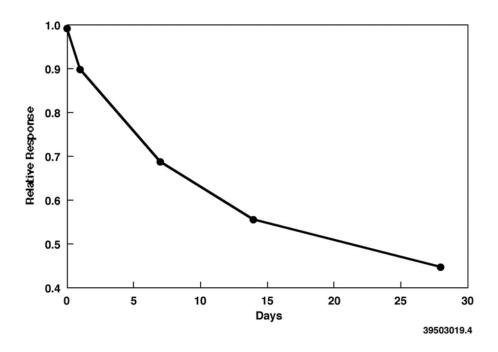
**Figure 5.15.** HSD Fading at 80°C
