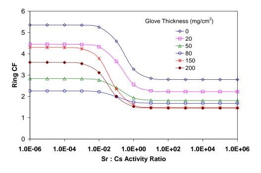
Figure 5.34 Ring Correction Factor as a Function of Sr:Cs Ratio for Large Area Source (on contact)
