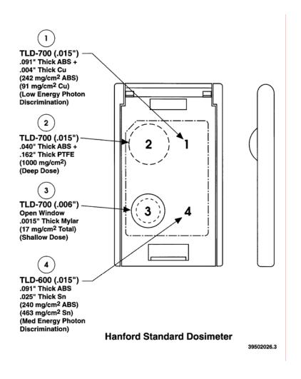
Figure 5.7 Hanford Standard Dosimeter
