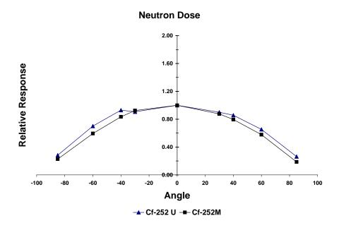
Figure 5.14. HSD Neutron Angular Response – Vertical Rotation
