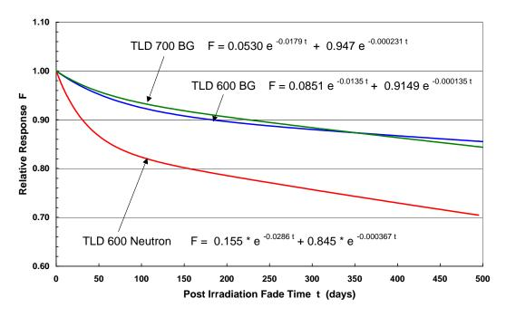
Figure 5.3 Post Irradiation Fade Functions Used for Hanford Dosimetry Materials
