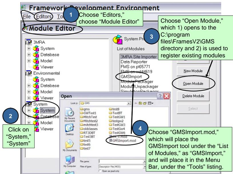
**Figure 4.3.** Steps for Registering the GMS Import Tool
