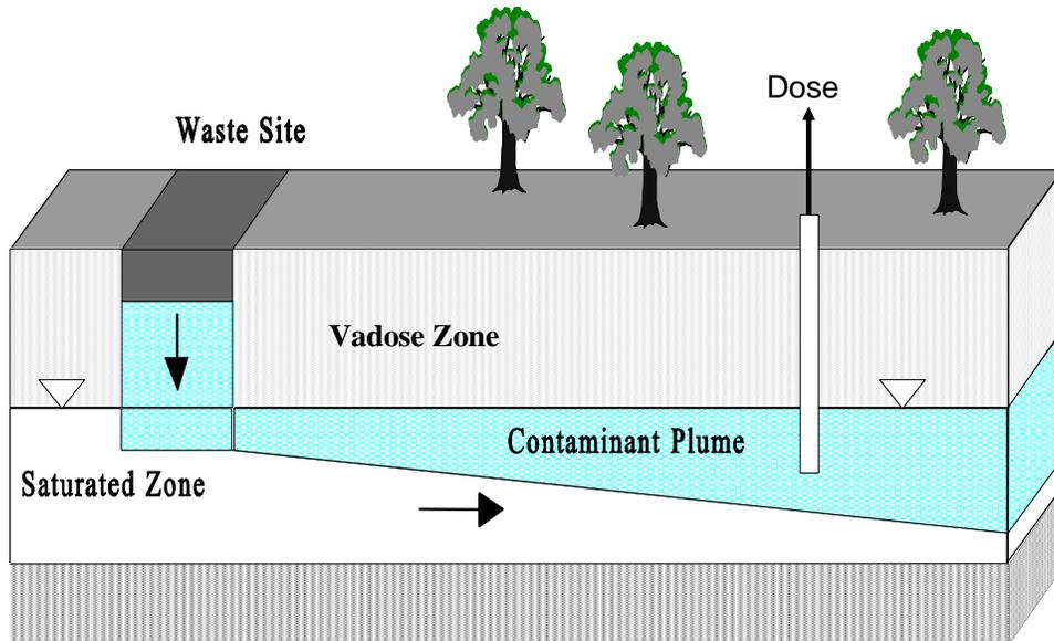
Figure 4.6. Illustrative Example of Aquifer Contamination
