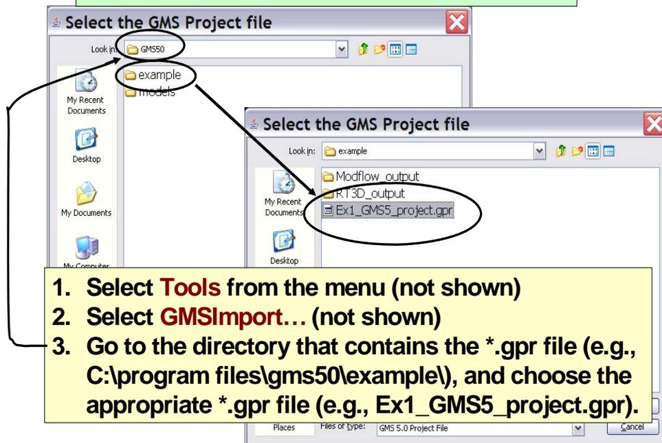
**Figure 4.4.** Steps for Registering the GMS Project File
