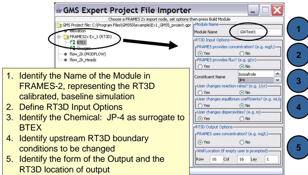
**Figure 4.5.** Steps for Defining How a GMS Module will Communicate with the User and FRAMES
