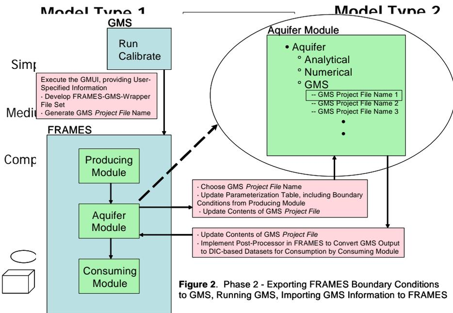
**Figure 2.** Phase 2 - Exporting FRAMES Boundary Conditions to GMS, Running GMS, Importing GMS Information to FRAMES
