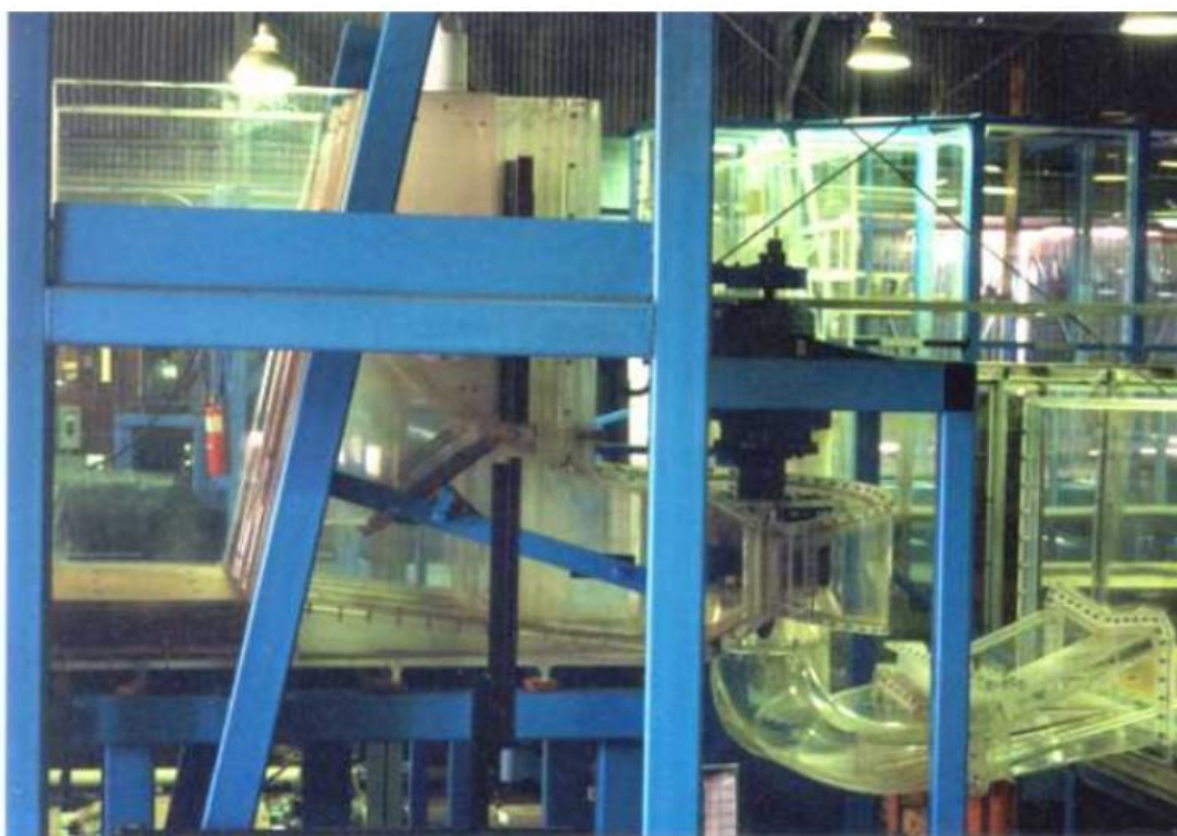
Figure 3.1. McNary Dam Observational Physical Model. The model is oriented with the immediate powerhouse forebay and turbine intake to the left and the turbine draft tube exiting into the tailrace to the right.
