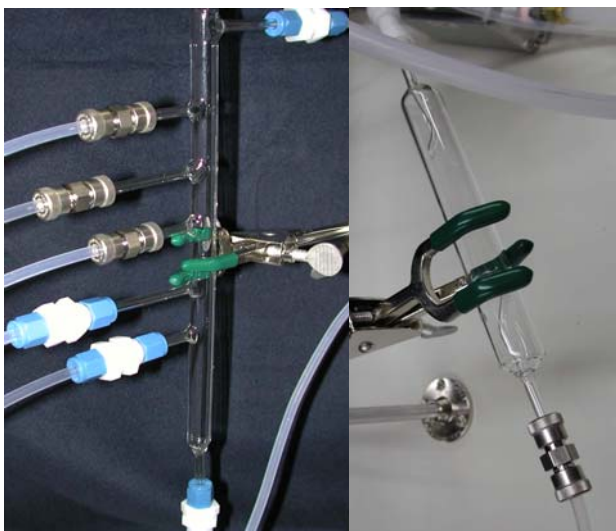
Figure 3.4. First Glass Manifold with Five Ports and Mixing Column
