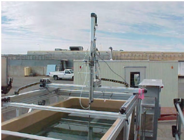
Figure 3.4. Gantry used to collect velocity measurements in the test facility.
