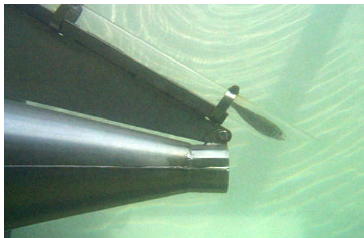
Figure 3.9. Fish release method just before entering the shear environment.
