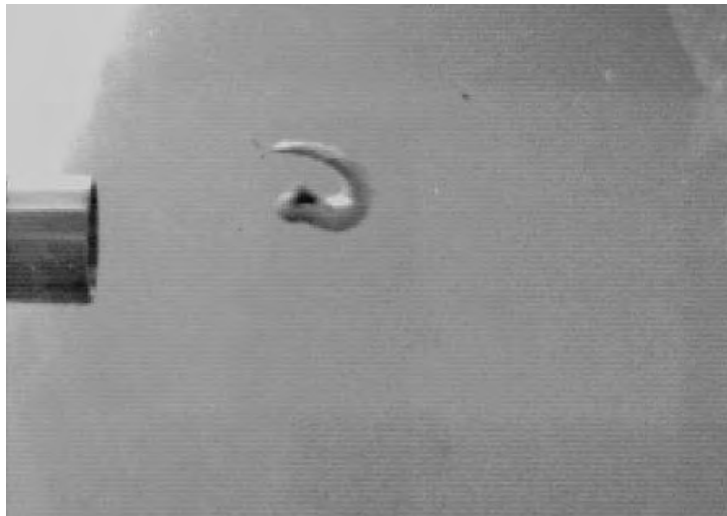
Figure 4.21. Digitized image of rainbow trout illustrating operculum flare upon exiting the nozzle during a fast-fish-to-slow-water test.
