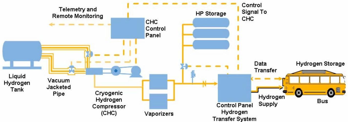
**Figure 5.1.** Hydrogen Fueling Facility
