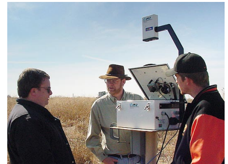
PNNL provides mentoring to users on specific instruments, such as this sky imager, at the ACRF sites.
