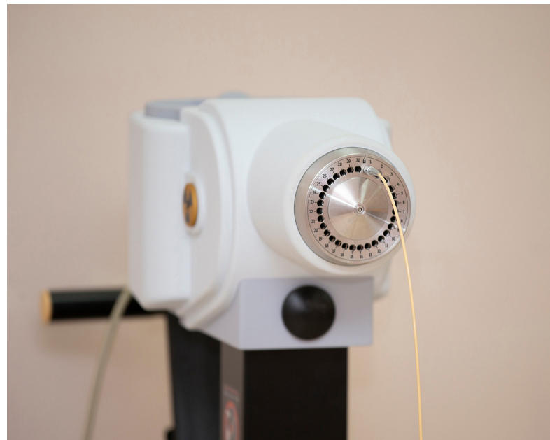
A high-dose rate afterloader used for treatment of prostate cancer using radioactive rays.
